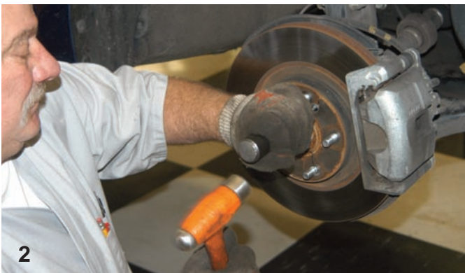
The two small screws that attach the rotor to the hub were disconnected. The screws are tight so they were broken loose with an impact screwdriver.
