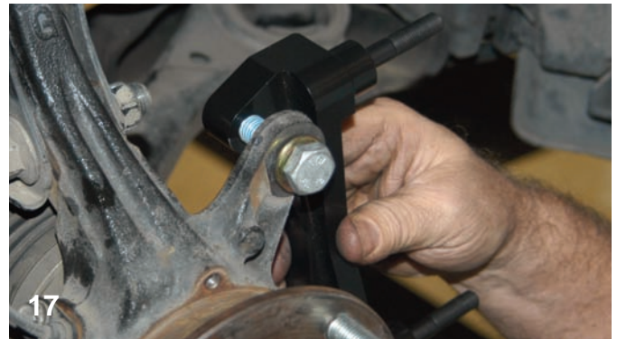
17 The bracket was held up to the original mounting ears and then the bolts were carefully screwed into the caliper bracket mounting holes.
