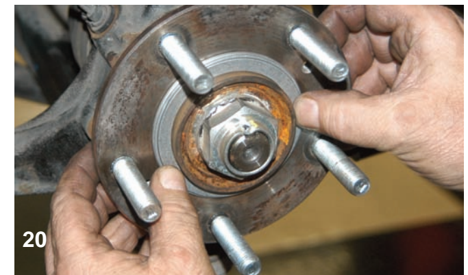
20 A spacer ring was attached to the centering ring to align the rotor assembly.
