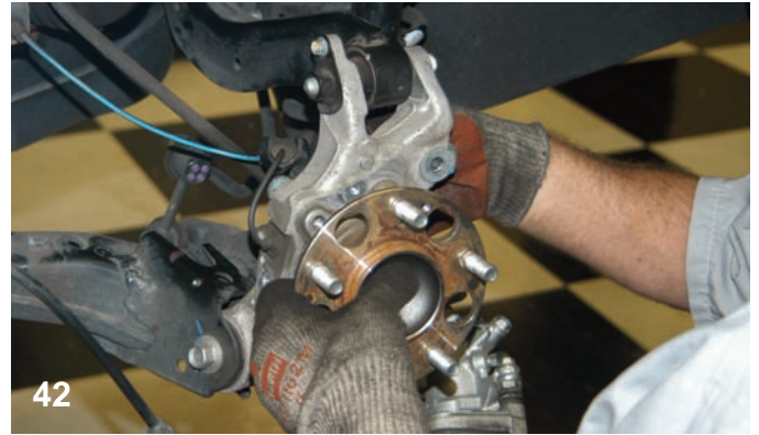
The hub assembly was reinstalled to the aluminum strut assembly using the original bolts.
