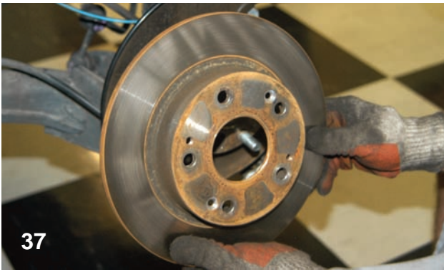
The rotor was removed from the hub assembly. This is a solid rotor that will be replaced by a vented rotor that is better in high heat situations.
