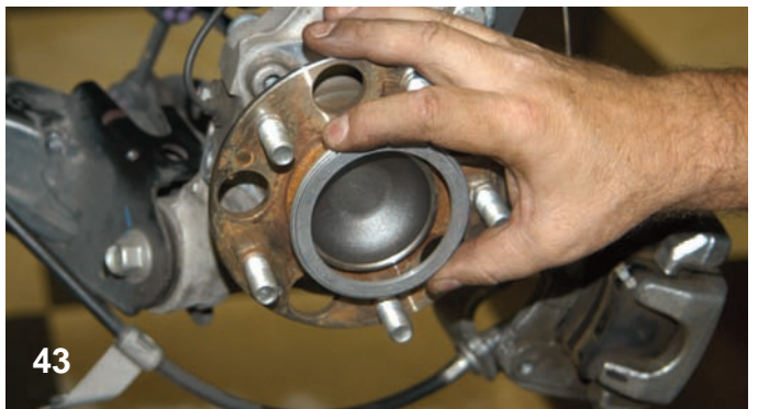
The centering ring spacer was installed over the centering ring. The spacer should be flush against the hub assembly.
