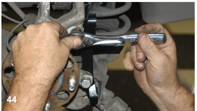
The caliper bracket was attached to the mounting ears using a socket wrench and the correct size socket. There should be a flat washer on the outside of the bolt and one shim washer between the mounting ears and the bracket.
