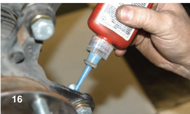
16 The caliper bracket bolts were coated with Loctite 271 before the bracket was installed permanently.
