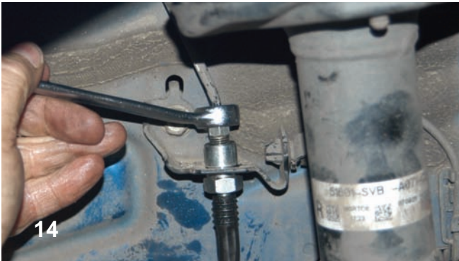
14 The Wilwood braided steel line and adapter were connected to the original hard line. It is important that all of the connections are tight to eliminate the chance for leaks.
