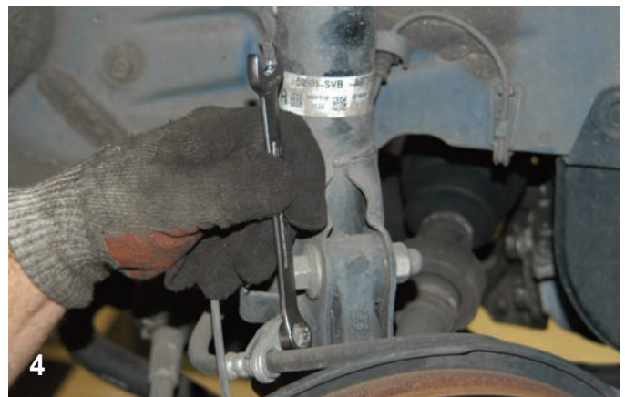
The original brake hose has a built-in bracket that connects to the spindle assembly. The bolt was removed followed by the caliper assembly.
