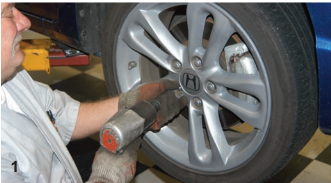
The Honda was elevated on a car lift, but this could also be done with a floor jack and jack stands. Using an impact Gun and the appropriated size socket, the lug nuts were disconnected in preparation for removing the wheels and tires.
