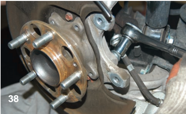
Using a socket wrench and the correct size socket, the bolts that secure the rear hub to the aluminum strut assembly were removed.
