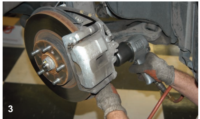
Using an impact gun and the appropriated size socket, the two caliper mounting bolts were removed.
