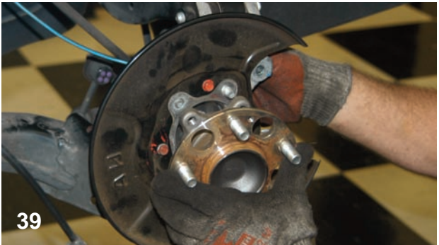
After the hub assembly bolts were disconnected, the hub was removed so that the rear dust shield could be removed.
