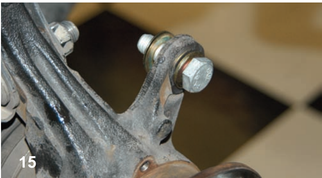
15 The caliper bracket has to be installed next. Here the bolts feature a washer on the outside and two shim washers on the inside. Shims can be added or subtracted to get the caliper centered over the rotor.
