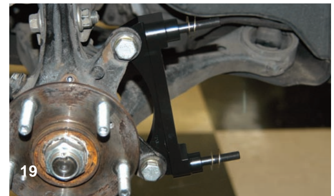
19 After the bracket is installed, two shim washers per stud were loaded on prior to installing the caliper.
