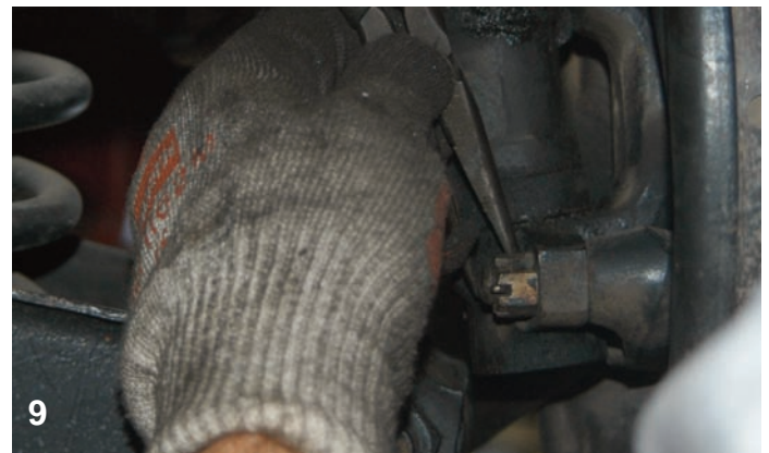
The backing plate is held on to the spindle with four nuts and bolts. First the cotter keys were removed from the nuts.
