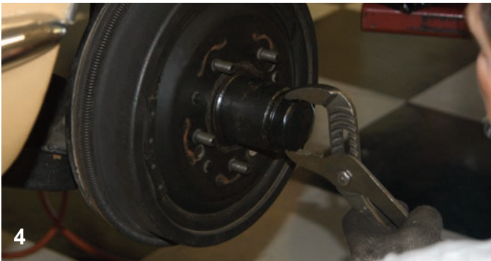
Removing the dust shield with channel lock pliers started the disassembly procedure.
