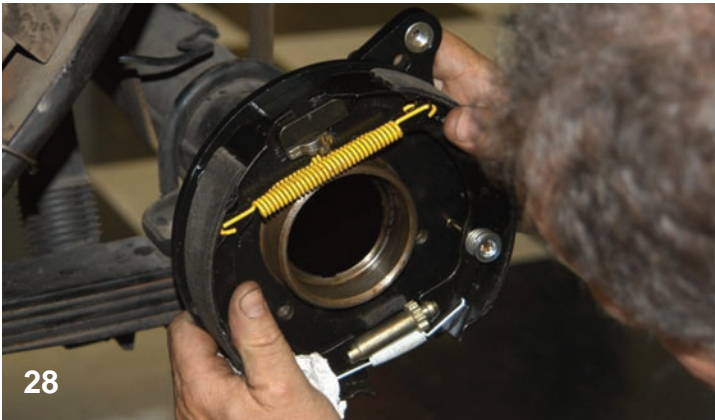
The Wilwood internal drum parking brake mechanism was installed on the axle and the holes in the unit were lined up with the holes in the axle flange. Notice that this unit is also equipped with the caliper bracket.
