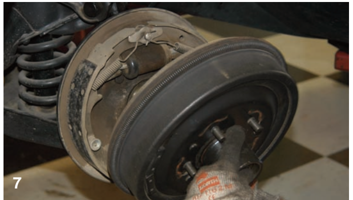
After the nut was disconnected, the brake assembly was removed from the spindle.
