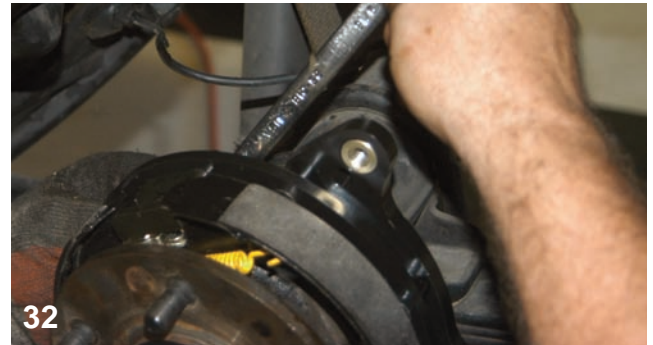
The four nuts were tightened with a box-end wrench. The nuts should be very tight.
