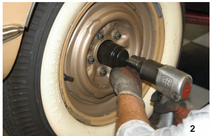
After the hubcaps were removed, the five lug nuts that secure the wheel to the brake drum were disconnected and then the tire and wheel were removed.
