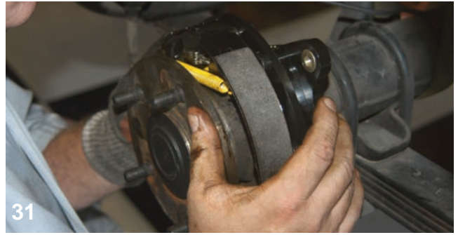
The axle was reinstalled, and the bearing retainer bolts were aligned with the holes in the internal drum parking brake unit and axle flange. The four bolts were installed at this time and then the nuts were started on the backside.
