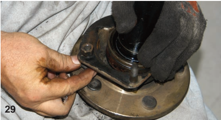
In order to get the axle back in place, at least two of the mounting bolts will have to be removed from the bearing retainer.
