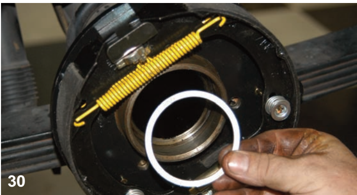
Before the axle is reinstalled, this small bearing spacer has to be installed in the axle.
