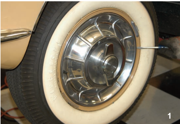
The original Corvette hubcaps were carefully removed by prying the edge up with a screwdriver.
