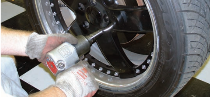
Using an impact gun and the proper size socket, the lug nuts were disconnected, and then the wheels and tires were removed.
