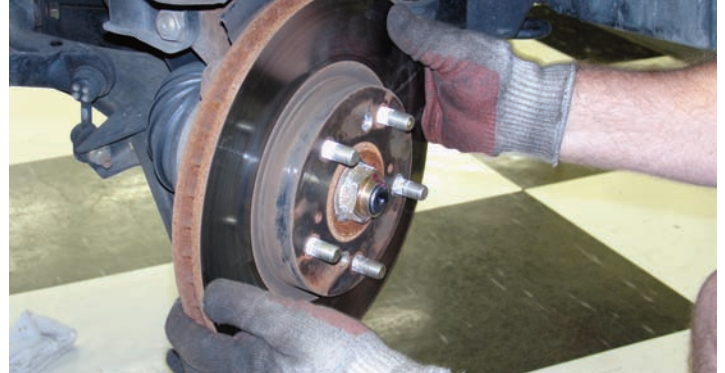
After the mounting screws were disconnected, the rotor was carefully removed from the assembly.
