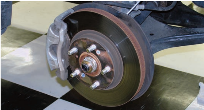
After the wheels and tires were removed, you can see the original Honda brake assembly. The Honda is equipped with a floating caliper.
