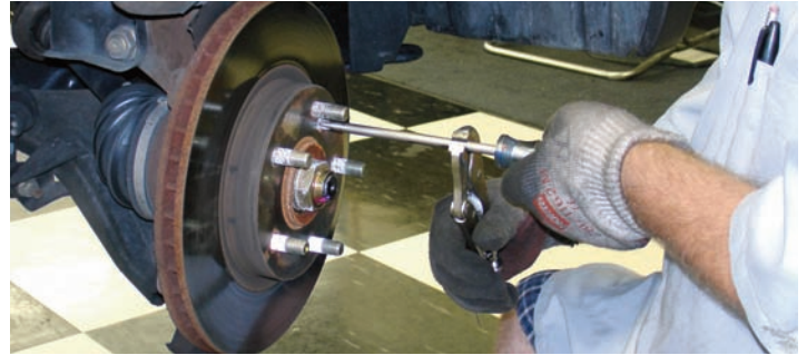
The screws that secure the rotor to the hub were removed with a screwdriver aided by lockjaw pliers. The screws are installed very tight.
