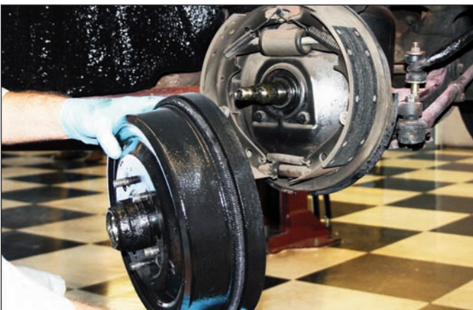
Sequence 3: Slide off the drum from the spindle. If it is stuck, it may be necessary to hit it a few times with a rubber mallet to break loose.
