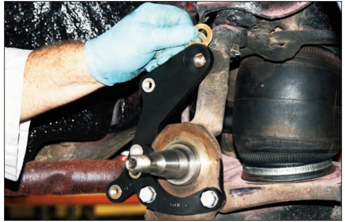
Sequence 10: The spindle bracket should initially be installed with clean, dry threads on the mounting bolts. Orient the bracket as shown and install using bolts, washers, and nuts. Place two shims between the bracket and upright on the top mounting bolt. Temporarily tighten the mounting nuts and bolt. NOTE: The bracket must fit squarely against the mounting points on the spindle. Inspect for interference from casting irregularities, machining ridges, burrs, etc. Grind spindle surface areas as necessary. Check that the bracket is aligned parallel to the rotor after sequence 18. If not, adjust by adding or subtracting shims between the spindle and bracket on the top bolt. Once the bracket alignment is correct, torque the lower bolt nuts to 47 ft-lb. Remove the upper bolt, apply red Loctite ® 271 to threads, and torque to 140 ft-lb. Remove, one at a time, the bolts that secure the bracket assembly to each other, apply red Loctite ® 271 to the threads and torque to 40 ft-lb.
