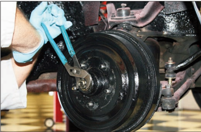
Sequence 2: Remove the dust cap and spindle nut retaining cotter pin. Remove the spindle nut.
