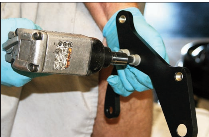
Sequence 9: Loosen the two bolts that secure the new caliper mounting brackets together so that the bolts are hand tight only.
