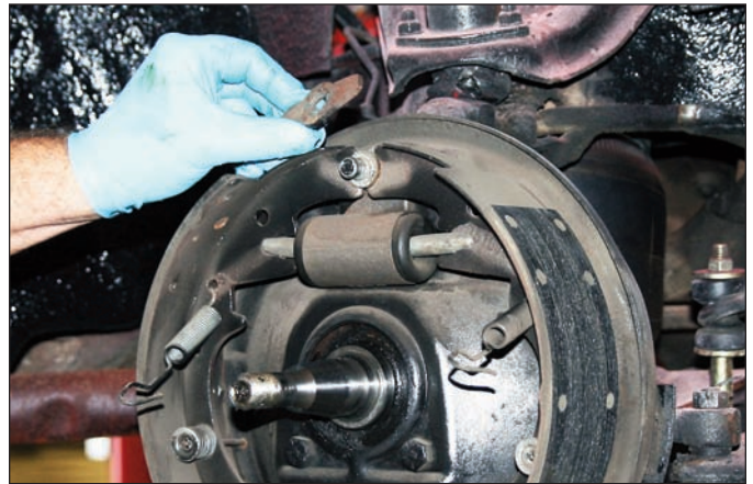
Sequence 5: Remove the lock clip over the bolt holding the brake assembly to the spindle.
