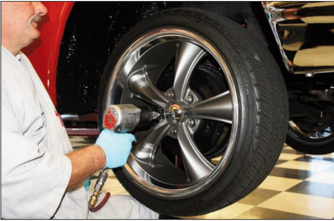
Sequence 1: Raise the front wheels off the ground and support the front suspension according to the vehicle's manufacturer's instructions. Remove the lug nuts, then lift off the wheel.
