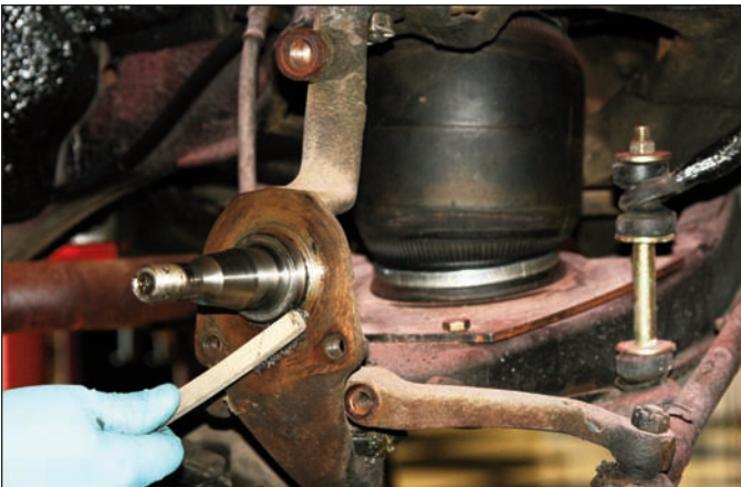
Sequence 8: Clean the spindle mount face and upright with a wire brush and remove any nicks, burrs, or grease that may interfere with installation of the new brake components.
