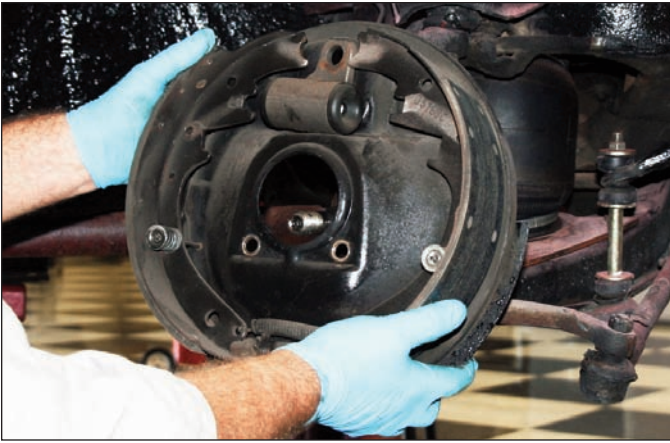
Sequence 7: Remove backing plate assembly while disconnecting the brake fluid hose.
