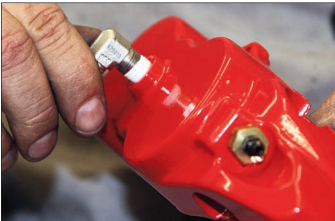
Sequence 21: Remove the protective sticker from the caliper fluid inlet. Coat the inlet fitting with PTFE thread tape and screw into the caliper with the 90° angle perpendicular to the length of the caliper.
