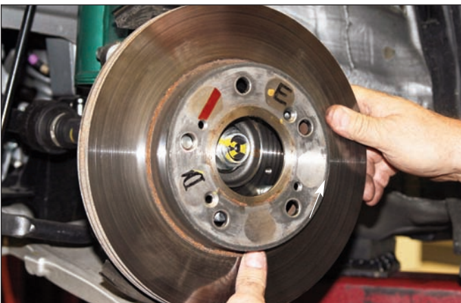
Sequence 9: Slide off the rotor from the hub. If it is stuck, it may be necessary to hit it a few times with a rubber mallet to break loose.
