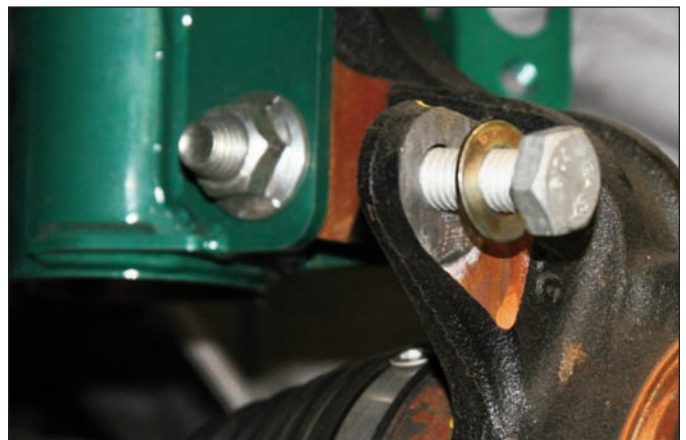
Sequence 12: Install the caliper mounting bracket bolt and washer from the outboard side of the caliper mounting ears.
