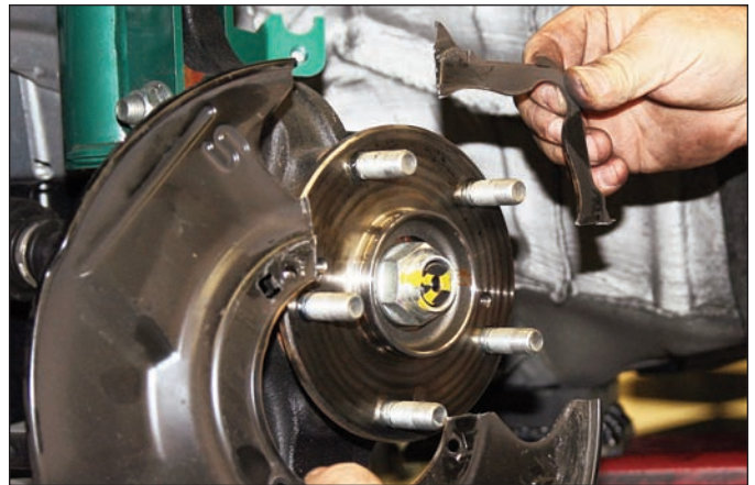
Sequence 11: Using a pair of tin shears, cut the dust shield at its two smallest diameter locations and pull apart. Remove and discard dust shield.
