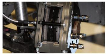
Looking from the top you can see the alignment of the rotor to the caliper and how the curve of the rotor matches the curve of the brake pads.
