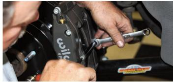
After the pads were in place, the bridge bolt was reinstalled and it was tightened with an Allen wrench and an open-end wrench.
