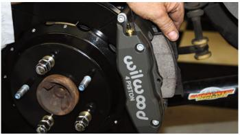
The bridge bolt was removed so that the BP-10 Smart Pads could be installed.
