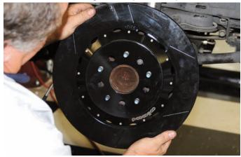
The large E-coated rotor was installed on the hub assembly. Notice the hub adapter is drilled with two mounting bolt patterns for the Chevy and for Ford, Chrysler, and AMC cars that all use the same lug pattern.
