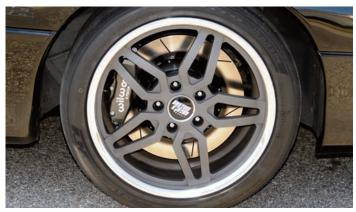
Here you can see the brake assembly through the spokes in the Camaro custom wheels. Notice that the pad bedding procedure cleaned the black coating off of the rotor face.
