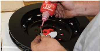
The small mounting bolts were loaded with a washer per bolt and then the bolts were coated with Loctite 271 before they were used to connect the rotor adapter to the rotor.
