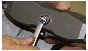
The fitting was tightened with a small open-end wrench. All of the hose connections should be as tight as possible to avoid brake fluid leaks.
