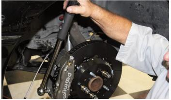
After the caliper mounting nuts were snug, they were tightened to 35 ft-lbs using a foot-pound torque wrench.
