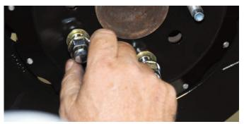
The rotor was connected to the hub assembly using three lug nuts. This will allow Tony to check the rotor to caliper centering to make sure it was the same as the other side.
