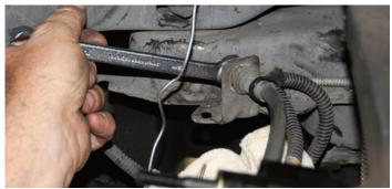
Using a line wrench, the connection between the steel hard line and the rubber flex line is disconnected.
