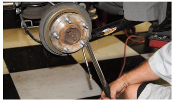
The caliper mounting bracket bolts were installed and then they were tightened to 75 ft-lbs using a foot-pound torque wrench.
