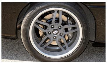
Here is the brake assembly seen though the spokes in the Camaro custom wheels. The nice feature of this kit is the front and rear calipers match in appearance, but the rear features four pistons to get the proper brake bias front to rear.
