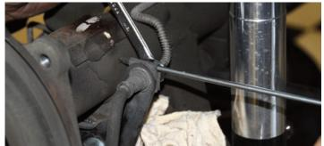
The spring clip was removed from the steel brake line to original hose assembly as seen here. After the clip was removed, the steel line to original hose connection was disconnected.
