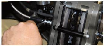
The Wilwood braided steel flex line was connected to the caliper inlet fitting. The aircraft-style line was super tight to make sure the connection was leak free.
