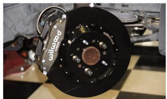
Here is the finished brake assembly with the large sixpiston Platinum-E coated Superlite caliper and the large 14-inch rotor. The face of the rotor is black now but after a few applications of the brakes it will go back to bare metal.
