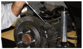
The caliper mounting bolts were very tight so they were disconnected with a large breaker bar.
