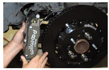
The caliper was placed over the studs and then it was lowered into place. This is a good time to check the caliper to rotor centering.
