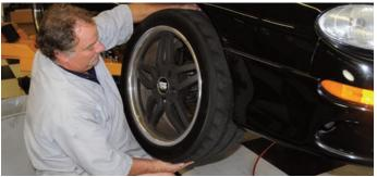
After the lug nuts were disconnected, the wheel and tire assembly was removed from the car and it was set aside for reinstallation later.
