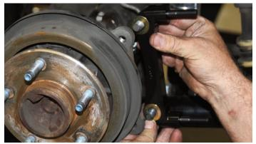
The caliper mounting brackets were installed to the original mounting ears. Notice the shim washer that is used between the bracket and the mounting ears.
