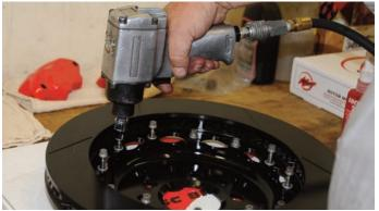
All of the rotor adapter bolts were tightened with an impact gun to get them snug.
