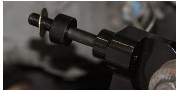
The mounting bracket for the caliper should be loaded with the spacer in the kit and the shim washer as seen here.
