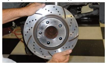
The aftermarket drilled and slotted rotor was removed from the hub assembly and it was set aside.
