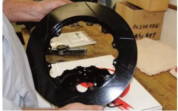
The E-coated 14-inch slotted rotor has to be connected to the hub adapter using the bolts in the kit.
