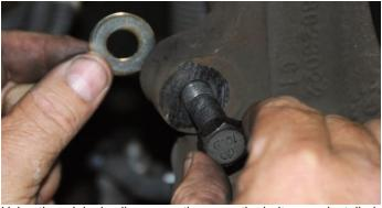
Using the original caliper mounting ears, the bolts were installed and one shim washer was installed between the ears and the caliper.
