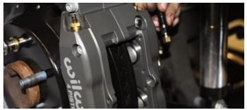
The Wilwood flex line was routed to the caliper and then it was attached. The hose should be very tight to avoid brake fluid leaks.
