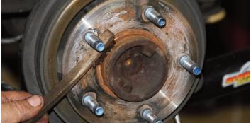
The face of the hub assembly was thoroughly cleaned with a wire brush.
