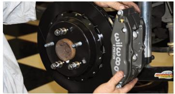
The Platinum-E coated four-piston Superlite caliper was carefully placed on the mounting studs.
