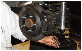
After the bolts were loose, they were disconnected using a small socket wrench. When the bolts were disconnected the caliper was removed.
