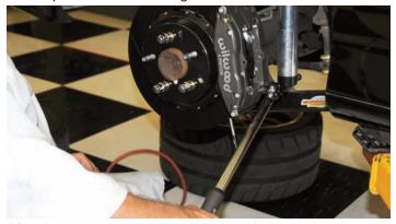
After the nuts were tightened down with the socket wrench they were tightened to 35 ft-lbs using a foot-pound torque wrench.
