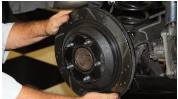
After the caliper was removed, the rotor assembly was removed from the hub assembly as seen here.
