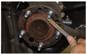
After the rotor was removed, the hub assembly was cleaned thoroughly with a wire brush.
