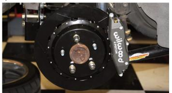
Here is the rear brake ready for action. The rear brake features the nice Platinum-E coated Superlite caliper and the large 12.90-inch rotor assembly. Now the brake assembly will need bleeding and pad bedding.
