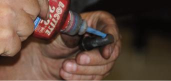
Before the bolts were connected to the caliper bracket, they were coated with Loctite 271 to keep them in place.
