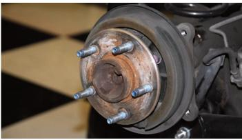
The Camaro uses a small drum-style parking brake assembly. The Wilwood rotor adapter was designed to work with this parking brake mechanism.
