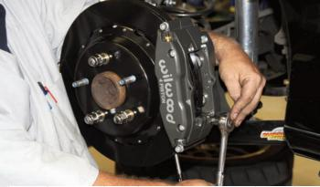
The washers were loaded on the mounting studs and then the locknuts were installed. After they were started by hand, the nuts were tightened with a socket wrench. At this point the caliper to rotor centering was determined.
