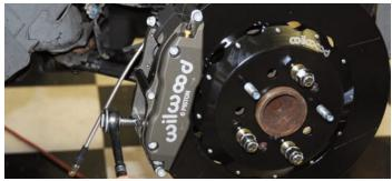
The washers and locknuts were connected to the mounting studs and then the nuts were tightened with a small socket wrench.
