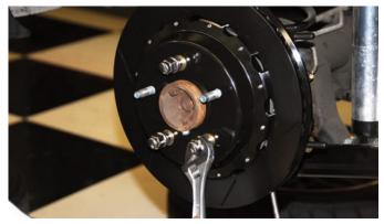
Three lug nuts were used to connect the rotor to the hub assembly. With the rotor on snugly, the rotor to caliper centering can be determined.
