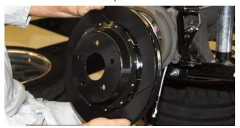
The rear rotor was assembled in the same manner as the front rotor. After it was assembled it was mounted on the rear hub assembly. This hub adapter works perfectly with the Camaro internal drum parking brake assembly.
