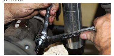
The Wilwood part number 220-9882 brake line was connected to the original steel line using the adapter fitting in the kit. After the hose was in place. it was secured to the bracket with a small spring clip.
