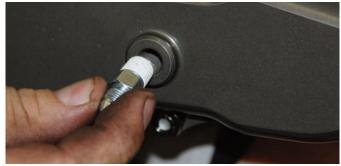
The caliper inlet fitting threads were coated with Teflon tape and then it was screwed into the caliper.
