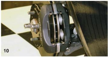
The two shims were perfect to get the calipers centered over the rotors. Here the two mounting bolts are snug in order to check the fit.
