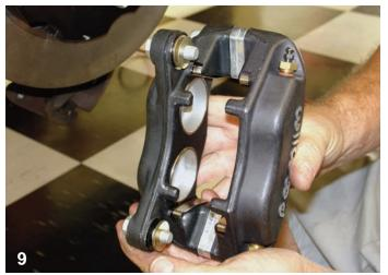
The caliper mounting bolts were placed through the Dynalite caliper mounting holes and then the bolts were loaded with two shims as seen here. Shims can be added or subtracted to make sure the caliper is centered over the rotor.
