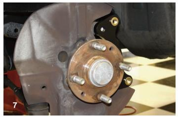
The mounting hub assembly should be thoroughly cleaned before the rotor is installed. Here a small rotor registration adapter was installed to help center the rotor on the hub. The smaller adapter diameter should be facing outward.
