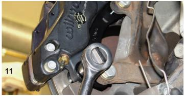
After the bolts were snug, they were coated with Loctite and then they were tightened to 40 ft-lbs using a foot-pound torque wrench.
