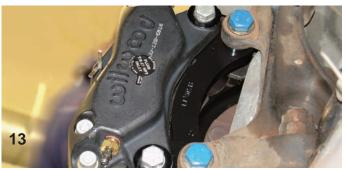
Under the round decal you will find the drilled hole for the hose adapter fitting. Remove the small decal and then install the fitting using PTFE Thread Tape on the threads. One end of the hose is attached to the fitting while the other end of the hose attaches to the steel hard line in the fender well.
