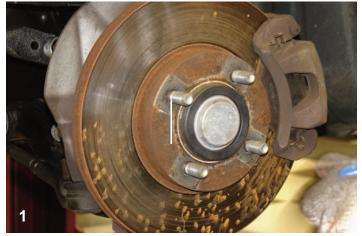
The original Miata brake uses a single piston floating caliper and a small rotor.
