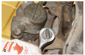
Using a socket wrench and the appropriate size socket, the original caliper bolts were disconnected and the caliper was removed.
