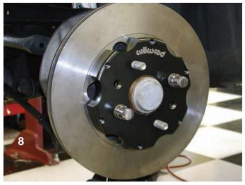
The rotor was installed on the hub assembly and then it was tightened with two lug nuts in preparation for finding the caliper to rotor centering.
