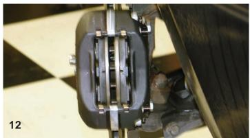
The brake pads were installed in the caliper and then the large cotter key was installed to keep the pads in place.
