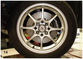
The wheel was reinstalled and now it is time for bleeding the brakes followed by the bedding procedure. The bedding procedure instructions can be found on the instruction sheet.
