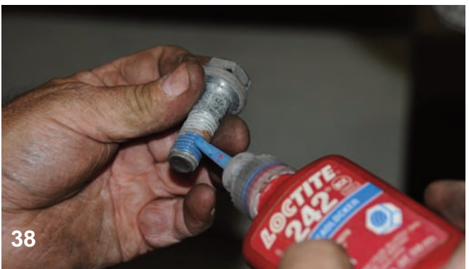
38 The original caliper bolts were reused and here they are being coated with Loctite 271. The original flat washer should also be retained.
