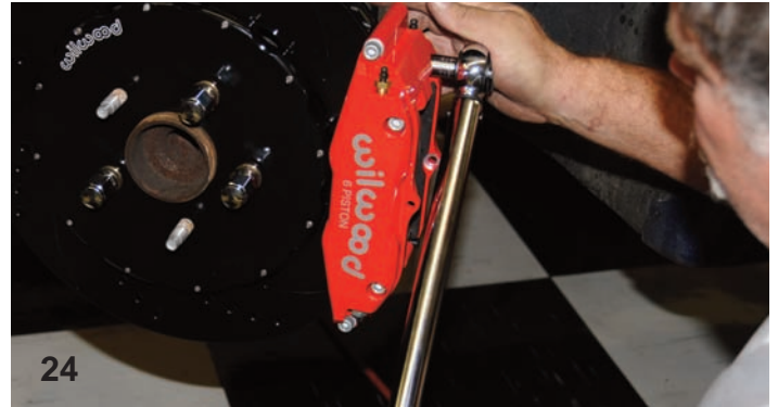
After the caliper mounting locknuts were snug, they were tightened to 35 ft-lbs using a foot-pound torque wrench.
