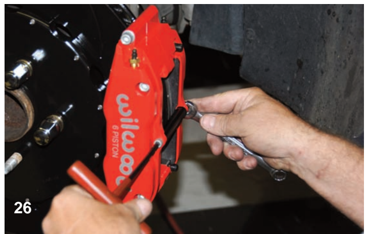
Using an Allen T-handle and an open-end wrench, the bridge bolt was tightened. A locknut is used to keep the bolt in place.
