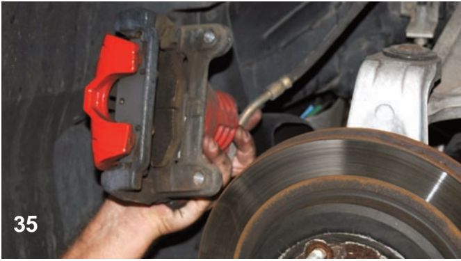
35 After the bolts were disconnected, the caliper was removed from the assembly.
