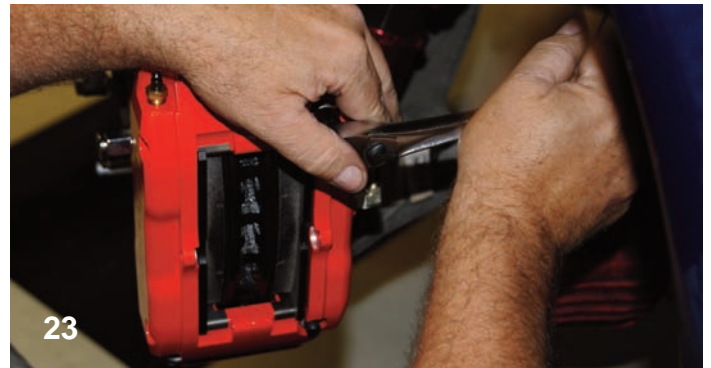
The caliper mounting nuts were tightened with a small socket wrench first.
