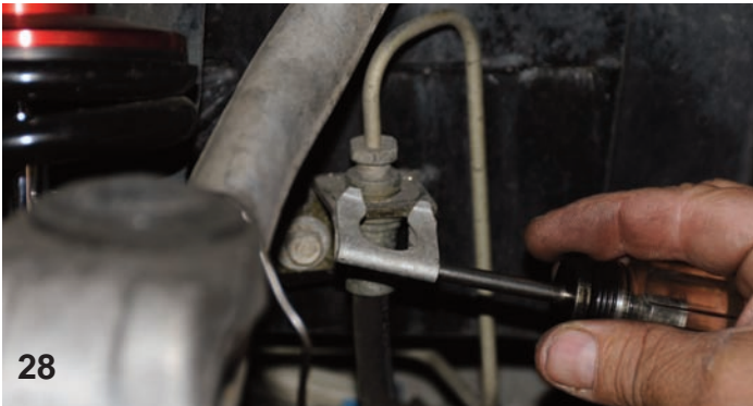
The spring clip that secures the flex line to the mounting bracket was disconnected.
