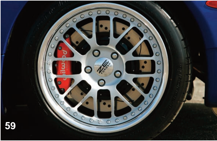
Here the rear brake assembly is finished and bedded in. The rear Superlite 4R calipers and 14-inch rotors match the front brakes adding to the aggressive appearance of the Corvette.
