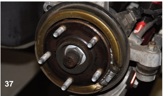
37 After the rotor was removed, you can see the internal parking brake assembly. The Wilwood rotors were designed to work with this system.
