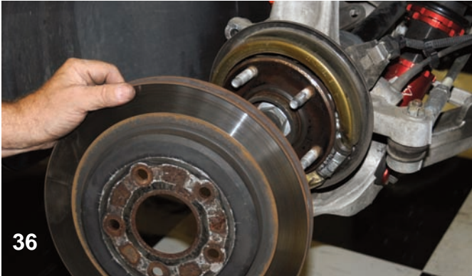
36 After the caliper was out of the way, the rotor was removed from the rear hub assembly.
