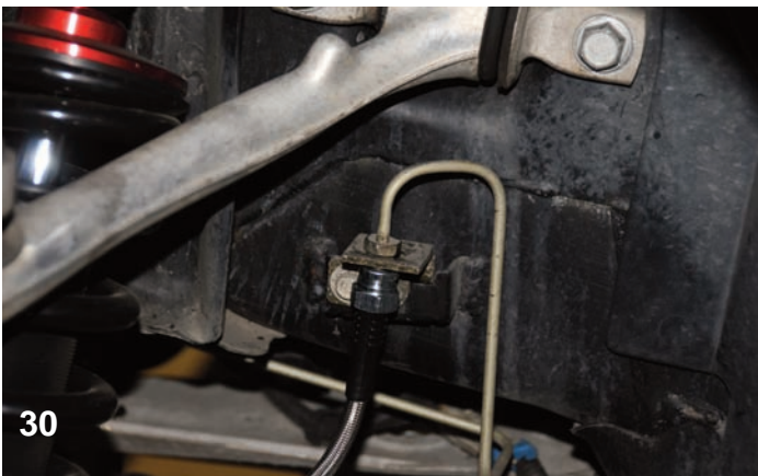
The other end of the braided steel Wilwood flex line was connected to the bracket and the original Corvette hard line.
