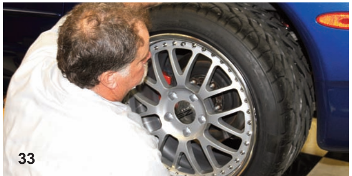
Here we see Tony removing the tire and wheel from the car so the brakes can be accessed.
