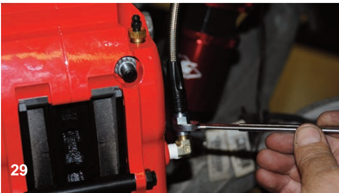
The Wilwood part number 220-8176 braided steel flex line was connected to the caliper inlet fitting using a line wrench.
