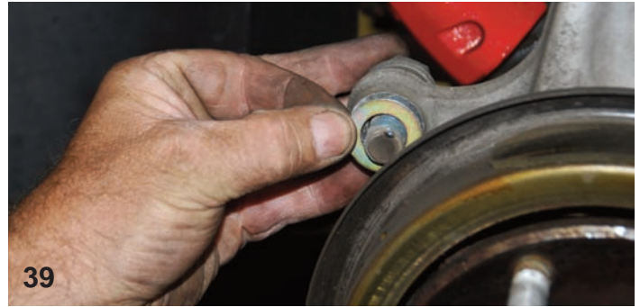
39 The original bolts were reinstalled into the mounting ears and a shim washer was installed. Adding or subtracting shims can be used to center the caliper over the rotor.
