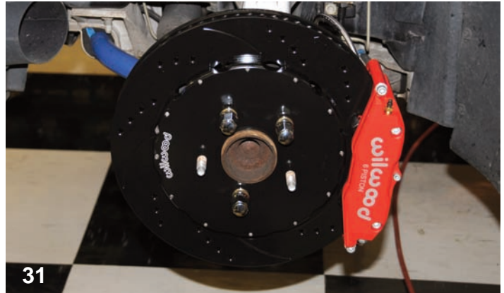
Here is the finished front Superlite 6R caliper ready for bleeding and bedding. After the bedding process is complete, the rotor face will be cleaned to shiny steel. The rest of the rotor that doesn't come in contact with the pad will remain covered with the black E-coating.
