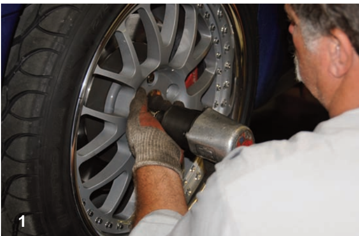
Using the appropriate size socket and an impact gun, the lug nuts were disconnected.
