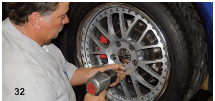
Using an impact gun and the appropriated size socket, the lug nuts were removed from the lug studs.
