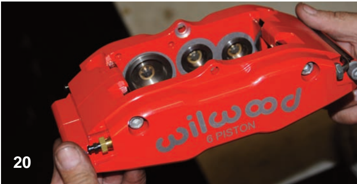
A look inside of the caliper shows that this unit was outfitted with Thermlock pistons, which are designed for high temperature track use.
