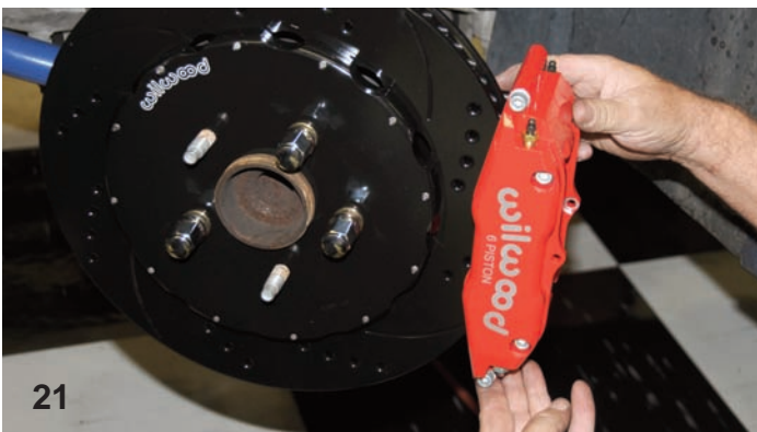
The calipers were installed into the studs and then the washers and locknuts were installed.
