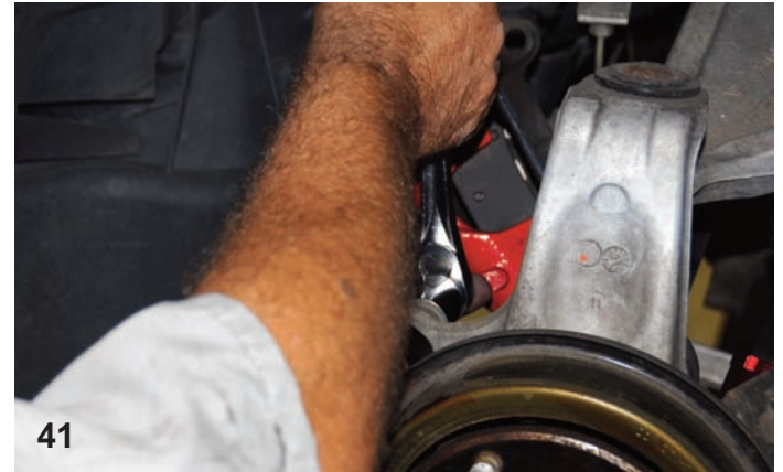
41 The upper bolt was also secured with a socket wrench as seen here.
