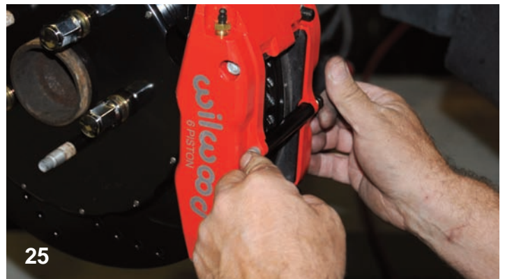
The caliper bridge bolt was installed to hold the brake pads in place. Here the bolt is being secured finger tight.
