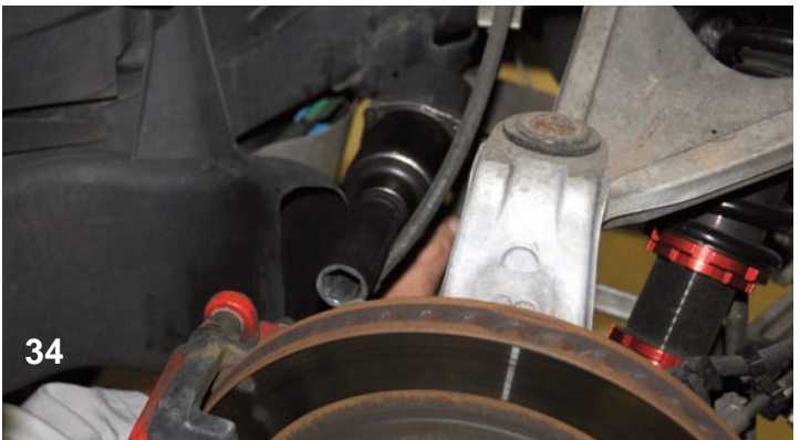
Using an impact gun and the appropriate size socket, the caliper bolts were disconnected.
