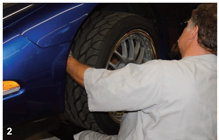
After the lug nuts were disconnected, the wheels and tires were removed. Here Tony is lifting the tire off of the lug studs.
