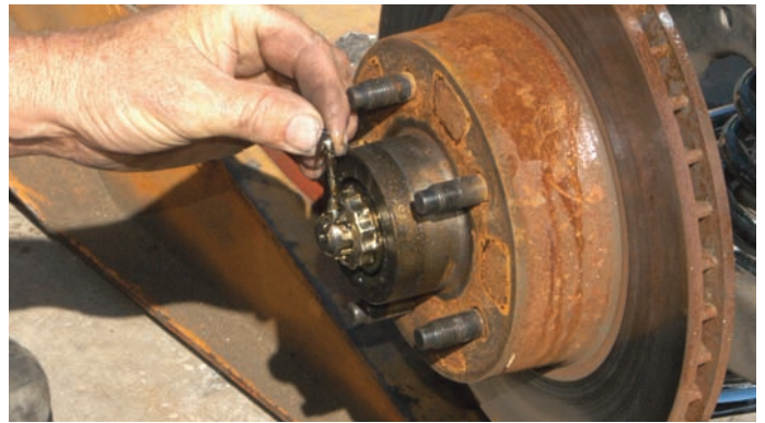
The cotter key was straightened out and then it was removed from the castle nut cover and spindle.
