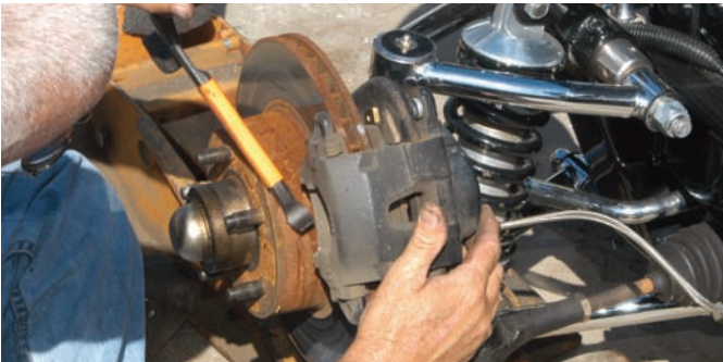
A small pry bar was used to separate the caliper from the bracket. When it was loose, the caliper was removed from the car. The brake line was still attached to the caliper so it was disconnected at the frame.
