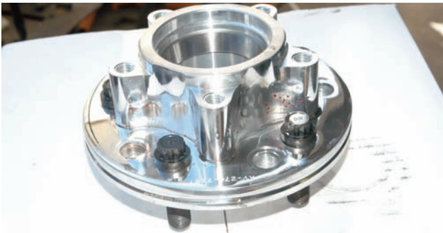
Here is the hub assembly after all of the bolts have been tightened. The hub is facing down because the adapter plate will have to be installed.
