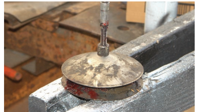
All four bearings were packed with high temperature disc break bearing grease using this bearing packer tool. If you don't have one of these in your toolbox, the bearings can be packed by hand but it takes a little longer.
