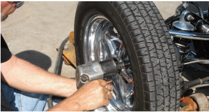
The car was elevated with a floor jack and stands were used underneath it as a safety feature. The lug nuts were removed with a 13/16-inch socket on an impact gun.
