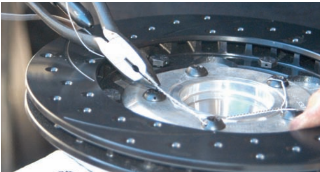
The E-coated rotor was attached to the hub adapter plate. The mounting tabs should be facing the outside of the hub assembly. The bolts were installed and then they were tightened to 22 ft-lbs. The bolts were tightened opposite of each other and after they all seem to be tight, the torque was checked a second time to be sure.
