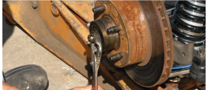
Using channel lock pliers, the large spindle nut was disconnected from the spindle. The nut, washer and castle nut cover were kept for the reassembly. The spindle nut could also be removed with a large Crescent wrench.
