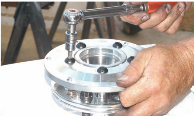
The hub adapter was secured to the hub assembly with the five button head Allen bolts as seen here. The bolts should be tightened to 180 in-lbs using an inch pound torque wrench. Notice that the dish is facing the front side of the hub.
