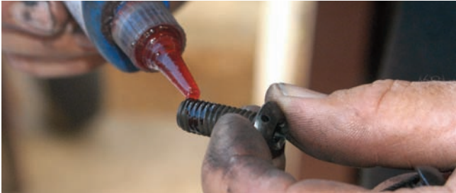
The five button head Allen bolts that secure the adapter to the hub assembly were coated with Loctite 271.
