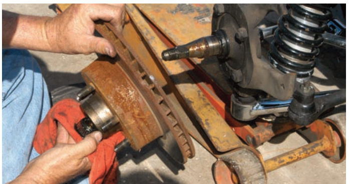
The rusty rotor was removed from the spindle. The non-coated cast iron rotor doesn't take long to rust and look terrible.
