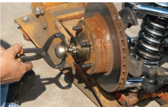
After the caliper was removed, the rotor could be removed. Here the dust cap is being separated from the rotor exposing the spindle nut assembly.
