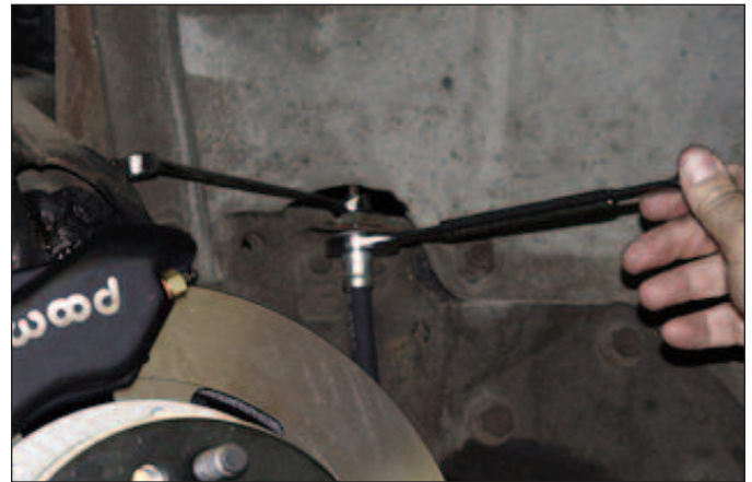
Sequence 23: Connect the other end of the flexline to the fitting at the brake hard line and install new clip. Secure line as necessary to prevent contact with moving suspension, brake, or wheel components. Bleed the system referring to the additional information in the data sheet as necessary for proper bleeding instructions.
