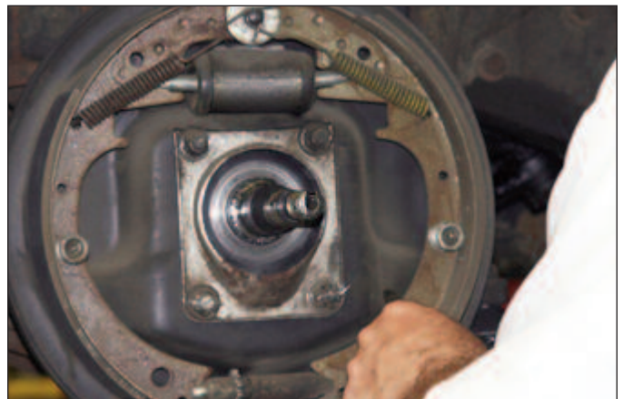
Sequence 6: Straighten and remove the two cotter pins that secure the two bottom bolts holding in place the drum brake assembly and steering arm.
