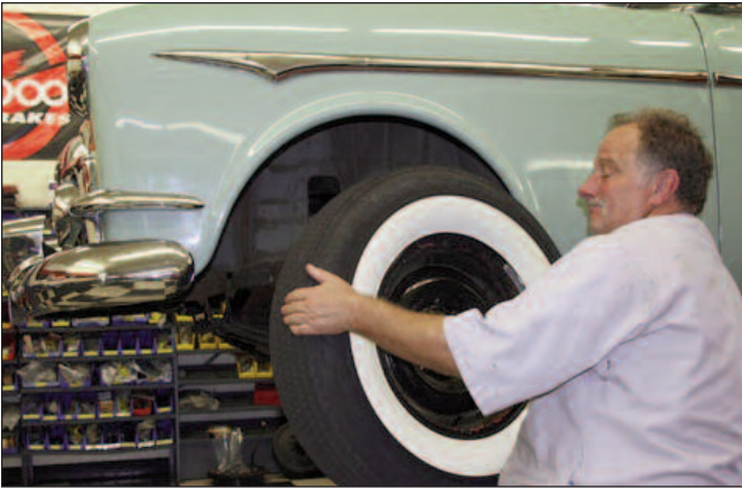
Sequence 1: Raise the front wheels off the ground and support the front suspension according to the vehicle's manufacturer's instructions. Remove the lug nuts, and then slide off the wheel.
