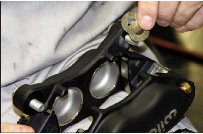
Sequence 19: Initially place two shim washers on each bolt between caliper mounting tab and the mounting ears on the bracket.
