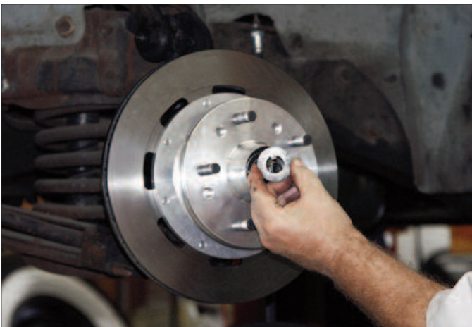
Sequence 15: Grease the non-threaded portion of the spindle and slide on the Rotor/Hub assembly. Install the indexed spindle washer, and castle nut.
