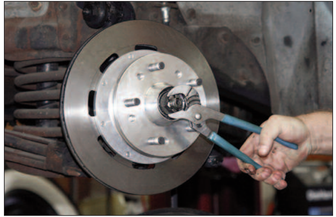
Sequence 16: Install spindle nut. Adjust bearings by tightening the wheel bearing nut to 60 in-lbs. while turning the hub/rotor assembly. Back off the adjusting nut one slot and install a new cotter pin (not supplied). The resulting adjustment should be zero (no pre-load to 0.003 inch end play).
