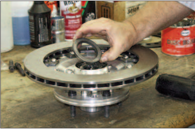
Sequence 13: Install the bearing into the hub. Install the grease seal by pressing into the backside of the hub/rotor, flush with the end of the hub section.
