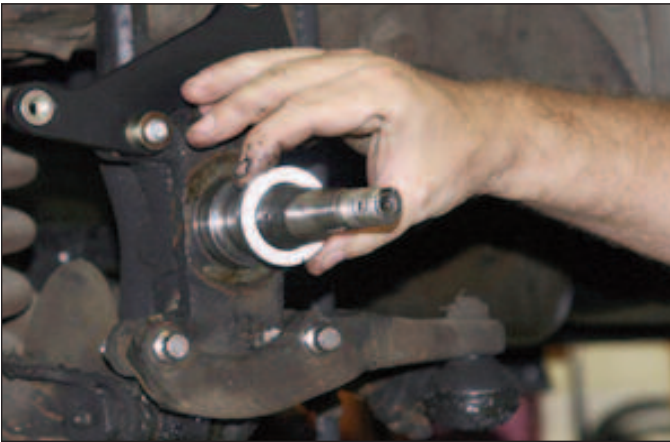
Sequence 14: Slide the hub/rotor spindle spacer onto the spindle being sure to have the chamfer edge inward.
