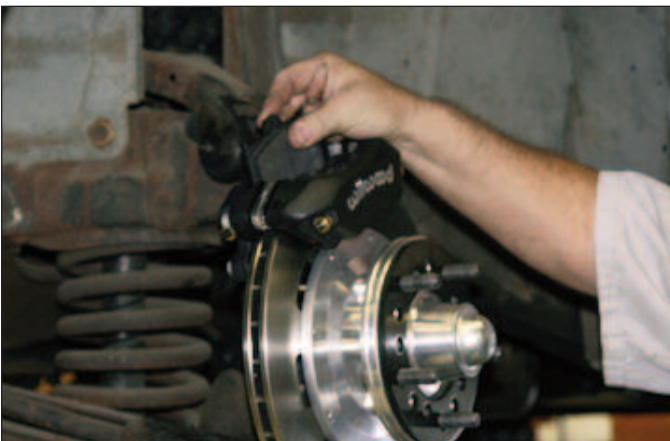
Sequence 21: Insert the brake pads into the caliper with the friction material facing the rotor.
