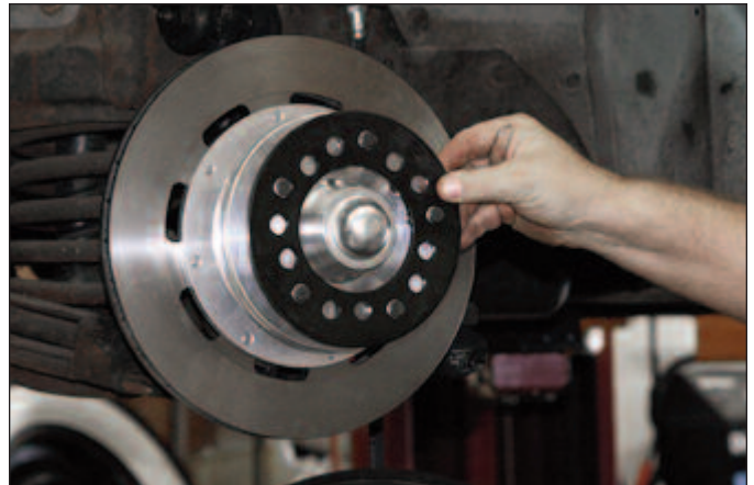
Sequence 17: Tap on the dust cover. Install the provided wheel spacer. This spacer provides the best matting surface between the hub and stock steel wheels.
