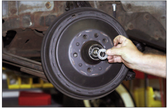
Sequence 4: Unscrew the spindle nut and remove the indexed retaining washer.
