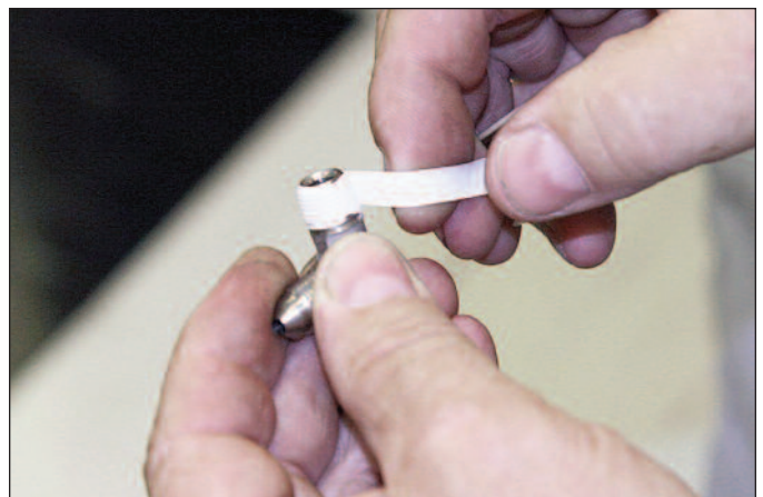
Sequence 18: Remove the protective sticker from the caliper fluid inlet. Wrap the inlet fitting with PTFE thread tape and screw into the caliper with the outlet facing rearward parallel with the caliper body.
