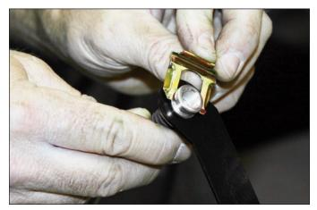
**Sequence 14**: Slip the new mounting bracket over the Wilwood flexline and secure with clip.
