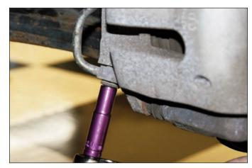
**Sequence 18**: Disconnect the other end of the rubber hose from the caliper. Try to keep fluid leakage to a minimum.
