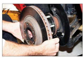
**Sequence 5**: Slide off the rotor from the hub. If it is stuck, it may be necessary to hit it a few times with a rubber mallet to break loose.
