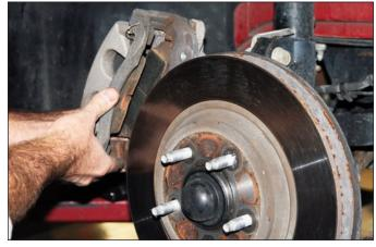
**Sequence 3**: Lift off the caliper and hang off to the side using a piece of wire.
