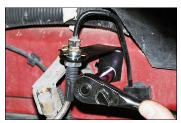
**Sequence 17**: Secure the new mounting bracket to the chassis using the saved OE bolt.
