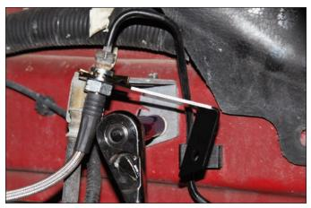
**Sequence 16**: Remove the old mounting bracket from the chassis. Save the mounting bolt.
