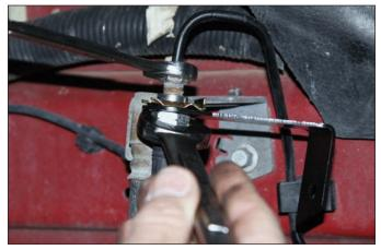
**Sequence 15**: Attach the Wilwood flexline to the brake hard line.
