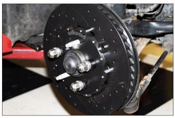
**Sequence 10**: Secure the hat/rotor with three lug nuts (finger tight) to keep the hat/rotor assembly in place while continuing with the installation.
