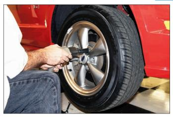
**Sequence 1**: Raise the front wheels off the ground and support the front suspension according to the vehicle manufacturer's instructions. Remove the lug nuts and lift off the wheel.
