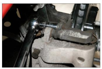
**Sequence 12**: Reinstall the caliper in its original location and torque the mounting bolts to manufacturer's specification.
