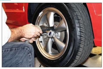
**Sequence 21**: Install the wheel and torque the lug nuts to manufacturer's specification. Rotate the wheel and check for any interference. Bed in the brake pads and rotor in a safe location before general use driving.
