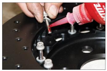
**Sequence 7**: Apply red *Loctite*<sup>®</sup> 271 to the mounting bolts and thread into the hat.
