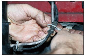
**Sequence 20**: Secure fluid line as necessary to prevent contact with moving suspension, brake, or wheel components. Bleed the system referring to the additional information in the data sheet as necessary for proper bleeding instructions.
