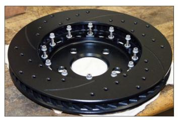
**Sequence 6**: The hat needs to be bolted to the rotor. Orient the rotor over the hat in the configuration shown above. Place one flat washer over each hole on the rotor mounting tabs.
