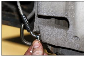
**Sequence 19**: Route line along the same path as the OEM hose and connect the other end of the flexline to the caliper.
