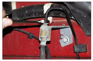
**Sequence 13**: Disconnect the OEM brake fluid hose where it connects to the brake hard line. Temporarily cap (not included) the line to minimize fluid loss.
