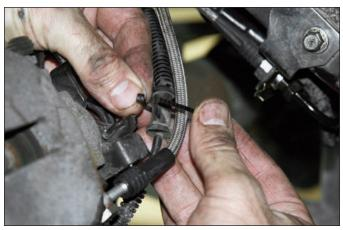
**Sequence 16**: Secure fluid line as necessary to prevent contact with moving suspension, brake, or wheel components. Bleed the system referring to the additional information in the data sheet as necessary for proper bleeding instructions.
