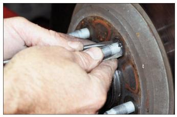
**Sequence 4**: Using a flat head screw driver pry off the rotor retaining washers from around the wheel studs.
