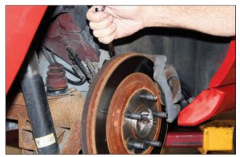
**Sequence 2**: Using a breaker bar and socket or wrench, break loose the caliper mounting bolts from the back side of the rotor.
