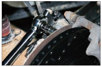
**Sequence 9**: Reinstall the caliper in its original location and torque the mounting bolts to manufacturer's specification.
