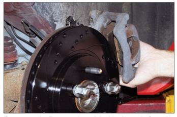
**Sequence 8**: Remove the original brake pads from the caliper and insert new Wilwood brake pads with the friction material facing the rotor.
