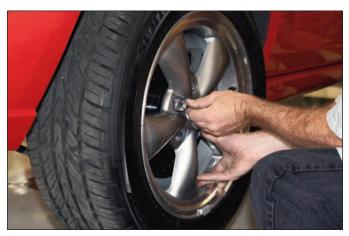
**Sequence 17**: Install the wheel and torque the lug nuts to manufacturer's specification. Rotate the wheel and check for any interference. Bed in the brake pads and rotor in a safe location before general use driving.
