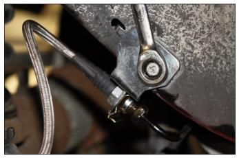
**Sequence 14**: Secure the new mounting bracket to the chassis using the saved OE bolt.
