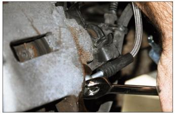
**Sequence 15**: Route line along the same path as the OEM hose and connect the other end of the flexline to the caliper.
