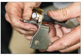
**Sequence 10**: Slip the new mounting bracket over the Wilwood flexline and secure with clip.
