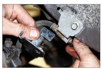
**Sequence 11**: Disconnect the OEM brake fluid hose where it connects to the brake hard line. Connect the new flexline to the hard line.
