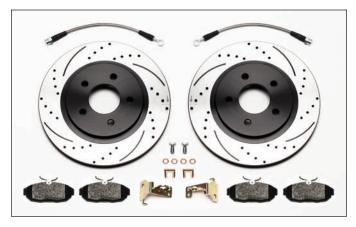
Wilwood part number 140-12149-D comes complete with SRP drilled and slotted integrated hat/rotors, ProMatrix brake pads and all necessary hardware for an easy bolton installation.
