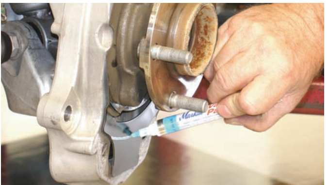
The dust shield will have to be trimmed, so a guideline was drawn where the metal will have to be removed.
