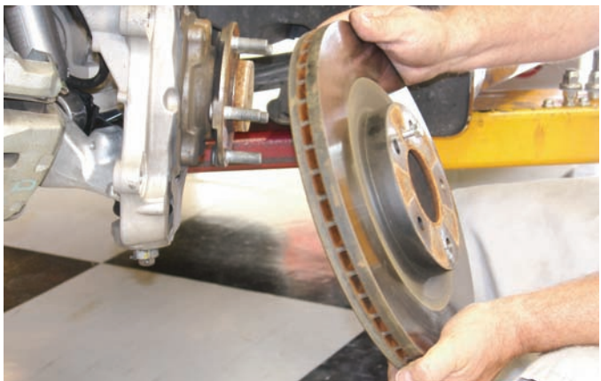
After the mounting bolt was disconnected, the rotor could be removed from the hub assembly.
