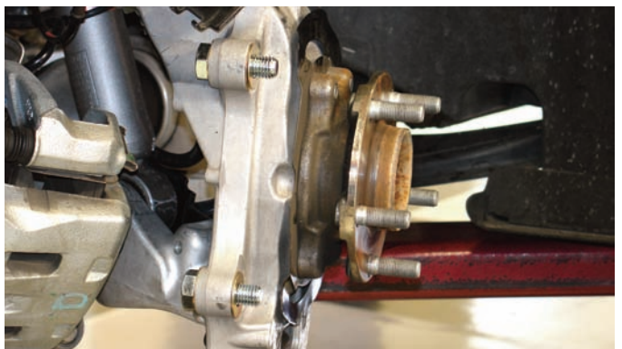
Here you can see the two caliper bracket bolts and washers loaded into the original caliper mounting ears.
