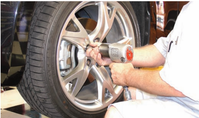
The car was elevated on a lift and then the lug nuts of the 19-inch diameter factory wheels were removed with an impact gun. After the nuts were disconnected the wheels were removed.
