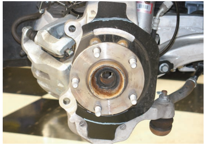
Here are the lines showing the two metal tabs that will have to be removed. The lines are used as a guide to follow when the cutting is being done.
