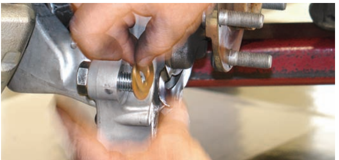
The caliper bracket mounting bolts were installed in the bracket ears and then they were loaded with two thin shim washers.
