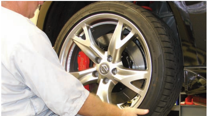
After the brakes were bled Tony installed the factory large diameter wheels and tires. The wheels were installed on the lug studs and then the lug nuts were installed and were tightened with an impact gun.
