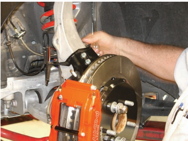
The Wilwood part number 220-9196 braided steel line was connected to the caliper inlet fitting and to the hard line connection on the other side of the upright.
