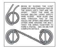
Figure 3. Safety Wire Diagram
