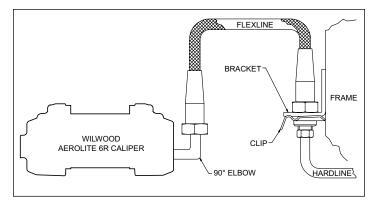
Figure 4. Brake Line Diagram
