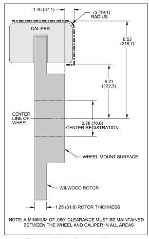
Figure 2. Wheel Clearance Diagram
