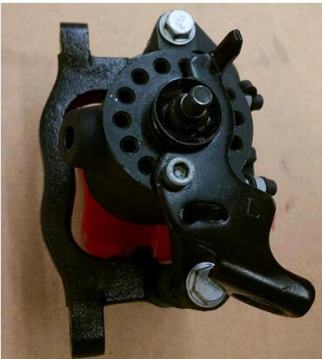
6) REINSTALL LEVER & TIGHTEN NUT (ALIGN SPLINES IN ARM TO SHAFT)
