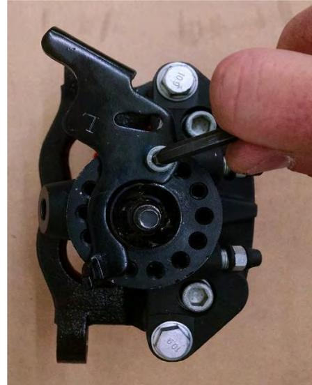
5) ROTATE ARM CLOCKWISE 7 (POSITIONS/HOLES) REINSTALL
