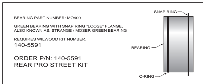
Figure 2. Loose Fit Flange Bearing Configuration
