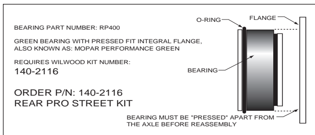
Figure 1. Press Fit Flange Bearing Configuration
