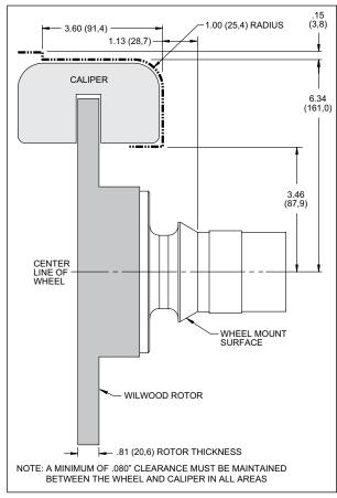
Figure 2. Wheel Clearance Diagram
