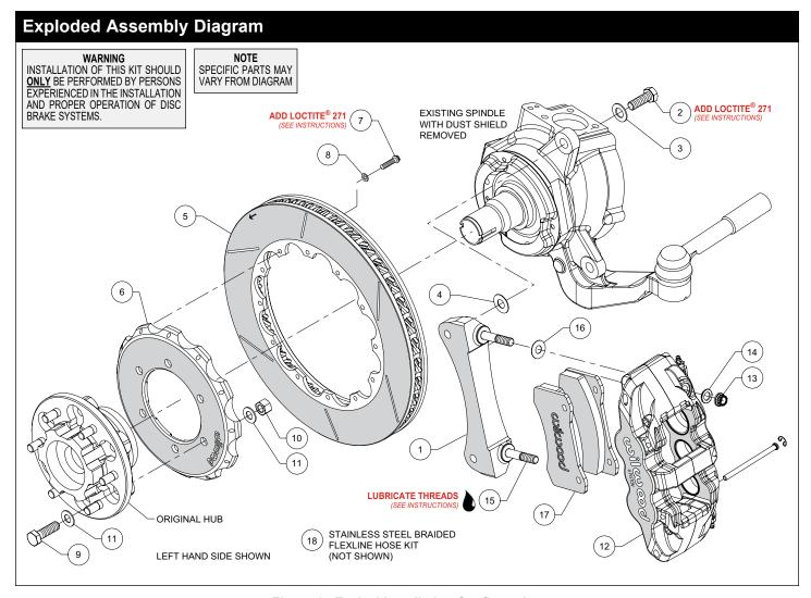
Figure 1. Typical Installation Configuration
