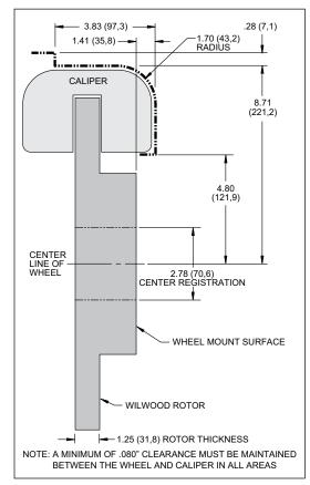
Figure 2. Wheel Clearance Diagram
