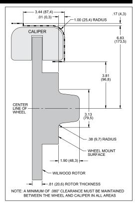
Figure 2. Wheel Clearance Diagram
