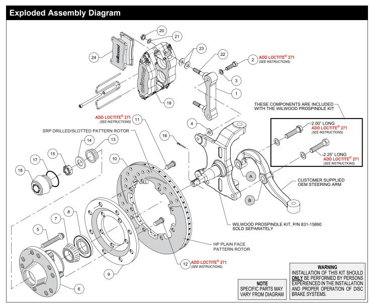
Figure 1. Typical Installation Configuration
