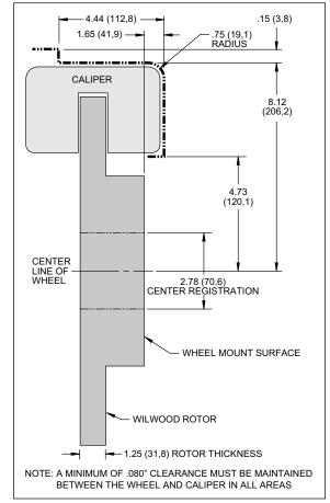
Figure 2. Wheel Clearance Diagram
