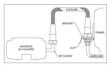
Figure 3. Brake Line Diagram
