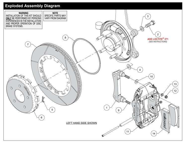
Figure 1. Typical Installation Configuration
