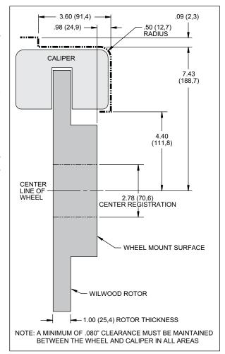
Figure 2. Wheel Clearance Diagram
