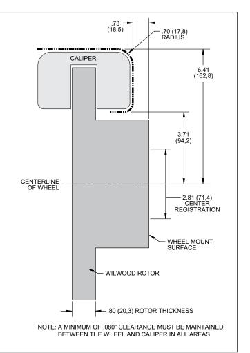
Figure 2. Wheel Clearance Diagram
