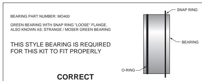
Figure 2. Loose Fit Bearing Configuration
