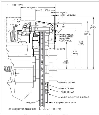
Figure 2. Wheel Clearance Diagram
