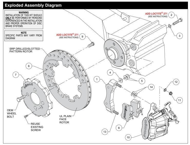
Figure 1. Typical Installation Configuration
