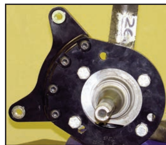
Photo 1 (4-Bolt Spindle Mounting)
