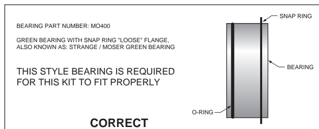
Figure 2. Loose Fit Bearing Configuration
