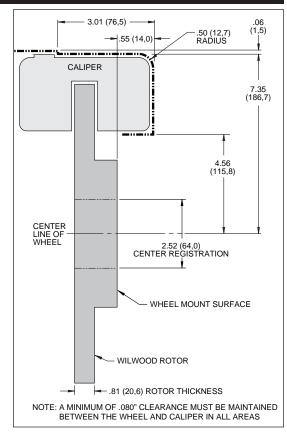
Figure 2. Wheel Clearance Diagram
