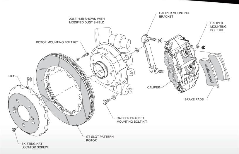
Figure 1. Typical Installation Diagram
