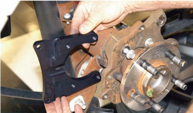
The intermediate caliper bracket was installed first as seen here.
