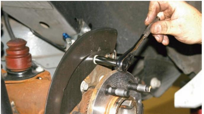
Using a small ratchet wrench and the appropriate size socket, the dust shield bolts were removed.
