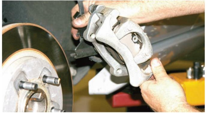
After the caliper bolts were removed, the heavy cast iron caliper was lifted up and was removed away from the car.
