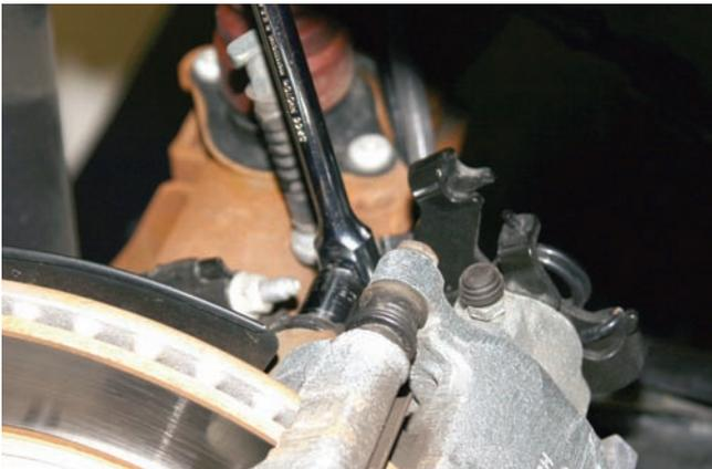
Using a ratchet wrench and the appropriate size socket, the caliper bolts and washers were removed.
