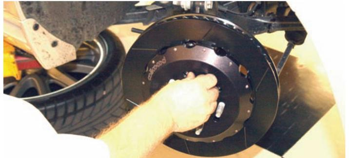
After the Wilwood caliper bracket was secured, the E-coated rotor was attached to the hub and spindle assembly.
