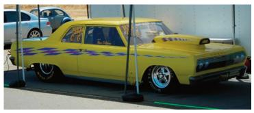
This early Chevelle was nice looking and it was definitely fast. This car runs a fiberglass front end for weight savings.
