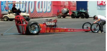
A very powerful fuel injected Ford Flathead engine powers this little dragster. The highly detailed car is a looker as well as a cooker.
