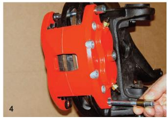
This view shows how the sleeve fits over the bolt and it will fit into the caliper body. The bolts screw in from the backside and the threads are close to the head of the bolt.
