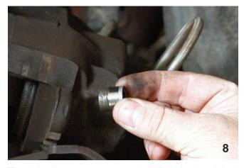
The old calipers were removed and here is the original sleeve. This one is worn out so it is a good idea to replace it with a new one.
