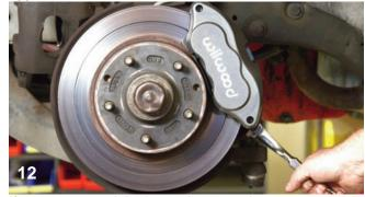
If you own an original muscle car and want to maintain a more original appearance you can upgrade the brake system by adding the gray (Platinum E) calipers, which are closer to the original color of the cast iron calipers. After the caliper is secured in place the flex line can be installed. You can use the original line but make sure you replace the copper crush washers. You can also upgrade the flex line by installing Wilwood part number 220-7056 lines to the banjo fittings and tighten.
