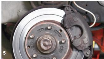
Here is the bake assembly after the tire and wheel were removed. Like we mentioned earlier, this would be the time to have the rotor surfaced if you find that it is necessary.
