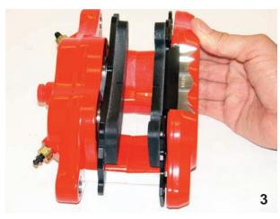
The pads fit into the caliper as seen here. The pads on the piston side are held in place by the bolts while the other side is held in place by the metal tab that fits into the caliper body. installation so you can decide if you have the mechanical ability to perform the installation or if you would prefer to have a mechanic do it for you.
