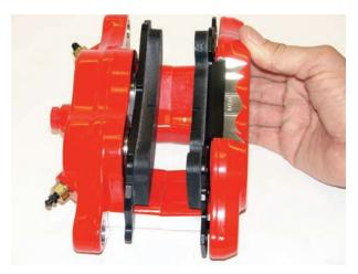
The pads fit into the caliper as seen here. The pads on the piston side are held in place by the bolts while the other side is held in place by the metal tab that fits into the caliper body. cide if you have the mechanical ability to perform the installation or if you would prefer to have a mechanic do it for you.
