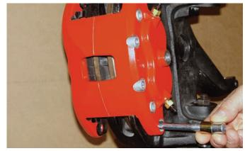
This view shows how the sleeve fits over the bolt and it will fit into the caliper body. The bolts screw in from the backside and the threads are close to the head of the bolt.
