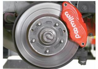
After the new calipers have been installed, the brakes will have to be bled to remove air from the lines. We installed the red caliper because it makes a nice appearance statement.
