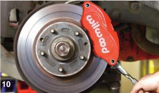
The Wilwood D52 caliper was installed by matching the mounting holes with the holes in the spindle bracket and then the two long Allen head slide bolts were installed. White grease should be applied to the slide portion of the bolts not the threads. At this point the banjo fitting can be installed making sure the threads are coated with PTFE thread tape. Also make sure the outside radius of the brake pad is aligned with the outside radius of the rotor face.
