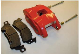
The D52 disc brake conversion kit comes with two calipers, BP-10 Smart Pads, the bolt sleeves and new Allen head bolts.
