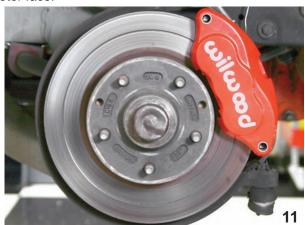
After the new calipers have been installed, the brakes will have to be bled to remove air from the lines. We installed the red caliper because it makes a nice appearance statement.
