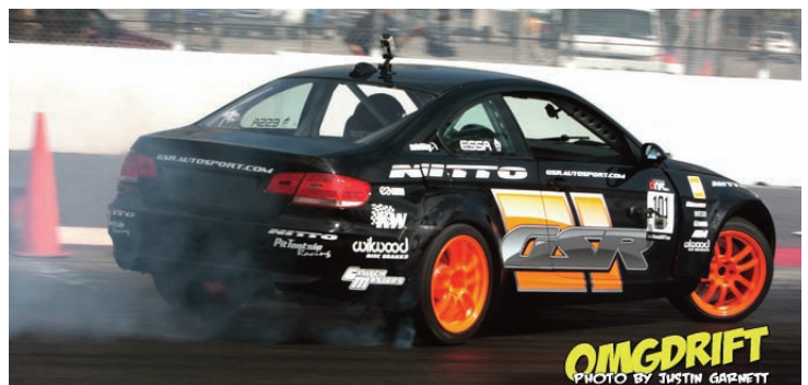
Michael Essa's new GSR Motorsports V10 powered BMW 335i grabbed a lot of attention all weekend. His BMW is set up with a custom 14-inch front kit with Wilwood Superlite calipers and twin rear Dynapros with a hydraulic handbrake.
