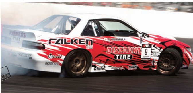
Dai Yoshihara looks to start the season off strong in his remodeled Falken Tire/ Discount Tire S13 that was built by SPD Metalworks and is powered by a 500+ horsepower LS6. Stopping comes in the form of lightweight Wilwood 13-inch rotors and Dynapro Calipers.
