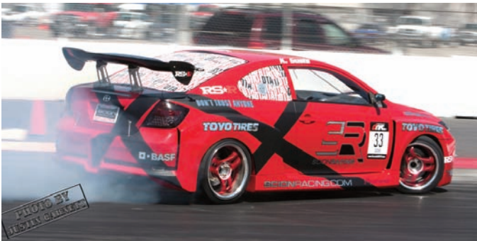
Ken Gushi attacked the course in his Scion Racing/RS-R TC. Ken's car is equipped with front Dynapro 6's with twin calipers in the rear including the Dynapro Single Hydraulic handbrake setup.
