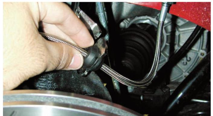
The original bracket outfitted with a rubber grommet directs the Wilwood line from the hard line to the caliper.
