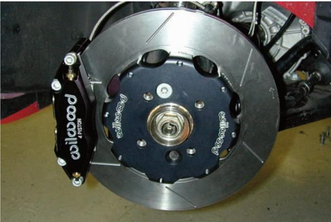
Here is the Wilwood Dynapro disc brake kit installed and ready for bleeding and bedding. This system features a four-piston caliper, a larger rotor and it is equipped with BP-10 Smart Pads for quick stopping power. The owner was very pleased with the brake improvement on the street and on the track.
