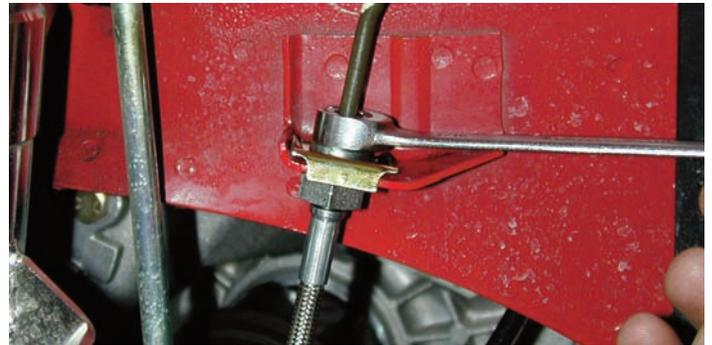
The Wilwood 220-8491 braided steel flexible line was connected to the original hard line using a line wrench.
