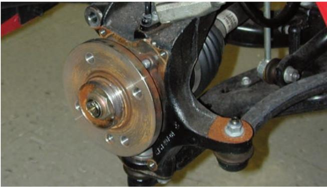
Here is the spindle and hub assembly after the dust shield was removed. Now it is easier to see the original mounting ears where the Wilwood caliper brackets will be attached.
