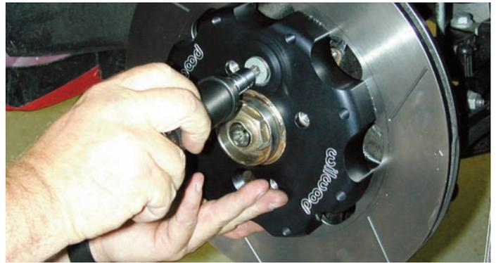
Using the original mounting screw the rotor was attached to the hub assembly.
