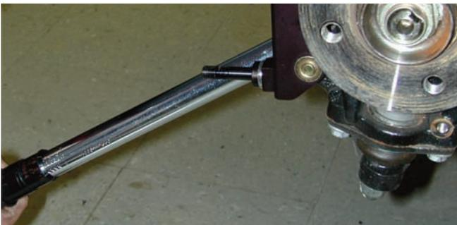
After the caliper to rotor spacing was correct, the bolts were coated with Loctite 271 and then the bolts were tightened to 75 ft-lbs using a foot-pound torque wrench.
