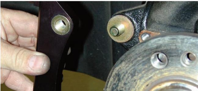
The mounting bolts were placed through the original caliper bracket and then they were loaded with two shims per bolt. The bracket was bolted on so the caliper to rotor spacing could be checked.
