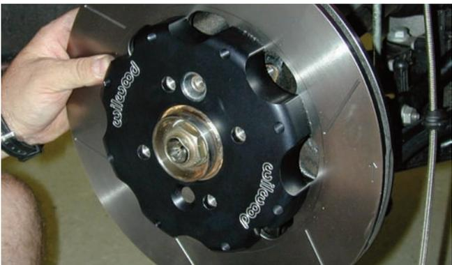
The adapter hat was bolted to the rotor using the bolts in the kit. The bolts should be coated with Loctite 271 and then the bolts should be tightened to 144 in-lbs. The rotor was then placed on the hub assembly.
