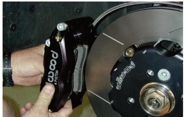
The caliper with the brake line installed was placed over the caliper mounting bracket studs. The centering was already checked so the pads were installed and the caliper was ready to be mounted permanently.
