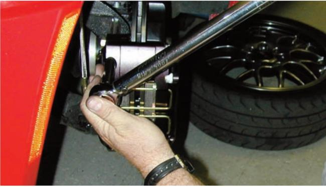
After the caliper was in place, the washers were installed and the two locknuts were tightened to 35 ft-lbs using a foot-pound torque wrench.
