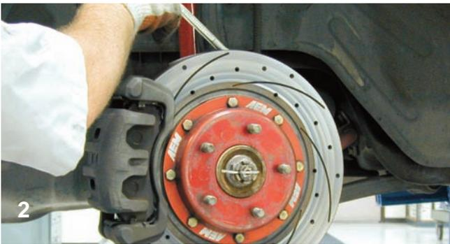
The caliper bolts were removed with a large breaker bar and then the caliper was disconnected. The rubber line from the caliper to the hard line should also be disconnected and the hard line should be capped until the new line is connected.
