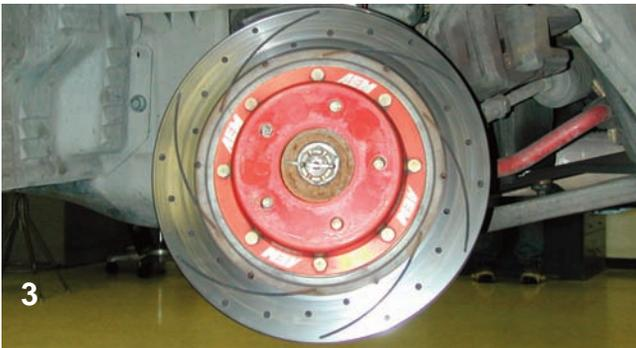
At this point the rotor can be removed from the hub assembly. Sometimes it is difficult to break it loose from the centering ring so it may need a few taps with a rubber mallet.
