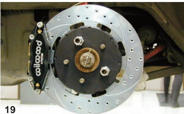
Here is the finished brake assembly featuring the DynaPro caliper and the slotted and drilled rotor. At this point the brakes will need bleeding and the pads to rotor should be bedded in following the directions on the instruction sheet.
