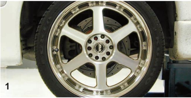
The front of the Eclipse was raised with a floor jack and was placed on jack stands. The lug nuts were disconnected with an impact gun and an appropriately sized socket, and then the wheels and tires were removed from the car.
