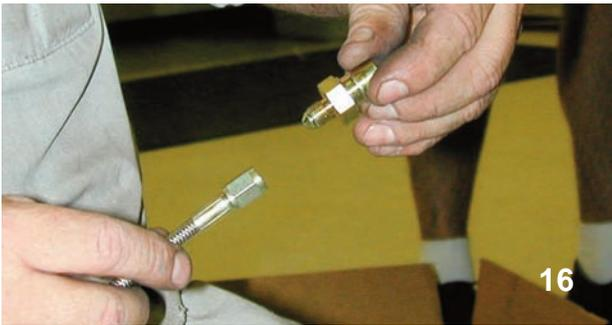
In order to connect the Wilwood part number 220-8293 braided steel hose to the original hard line this fitting must be used. Here the hose and fitting are being connected.
