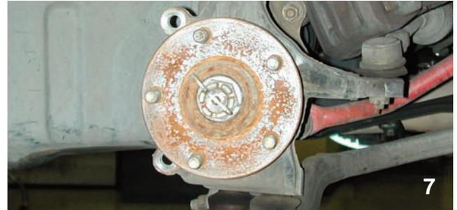
The hub assembly and the caliper mounting ears were cleaned with a wire brush prior to mounting the Wilwood caliper bracket.
