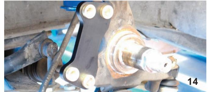
Here is the Wilwood caliper bracket after it was installed. The bracket was bolted on with two 1 1/2-inch long 7/16-20 bolts followed by a 0.063-inch thick washer. The bolt goes through a sleeve and on the other side of the spindle there is a small spacer and another 0.016-inch thick washer. Notice the curve on the inside of the bracket to allow clearance for the hub assembly.
