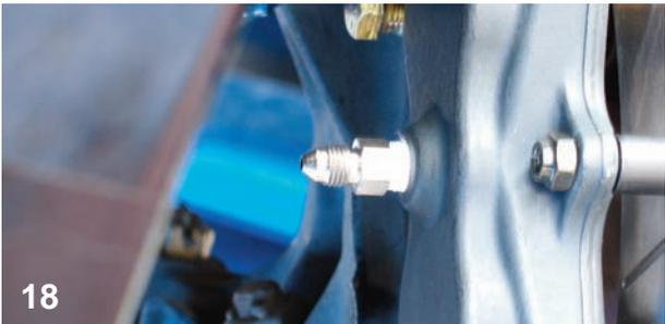
The inlet fitting threads were coated with PTFE thread tape and then the inlet fitting was screwed into the side of the caliper.
