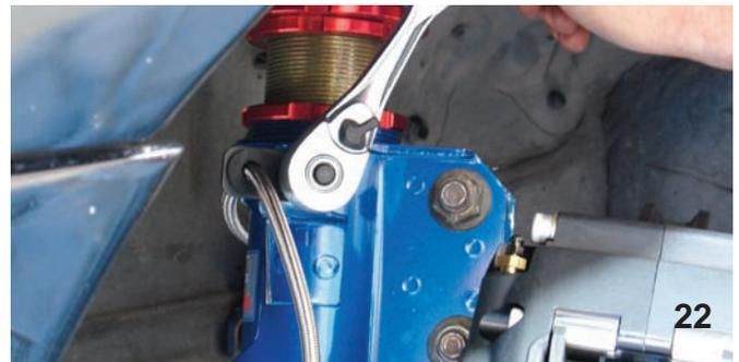
The Wilwood part number 220-9199 stainless steel line was secured to the strut with a small clip as seen here.
