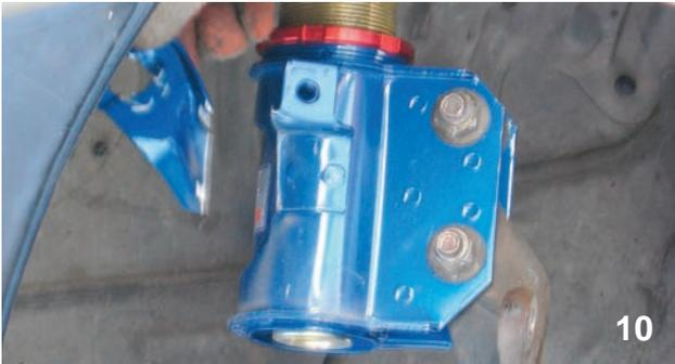
Using a small three-inch cut-off wheel, the bracket was removed from the strut assembly.
