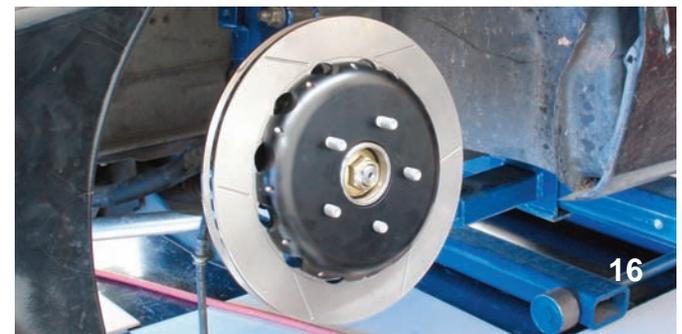
The Wilwood rotor was assembled before it was installed on the hub assembly. Using the small bolts and washers in the kit, the rotor was bolted to the hub assembly. The bolts were coated with Loctite 271 and then they were tightened in an alternating sequence to 85 in-lbs using an inch-pound torque wrench.
