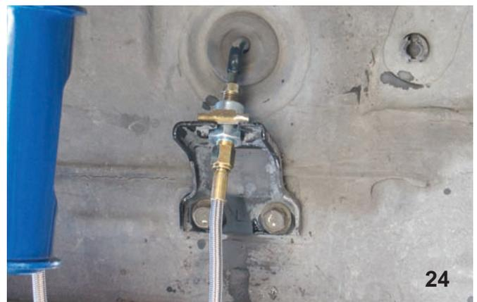
The other end of the stainless steel line was run to the original bracket that was outfitted with an adapter fitting that mates the original steel line to the Wilwood Flexline.
