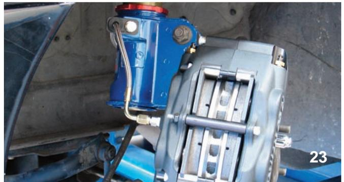
Here you can see the feed line running to the caliper mounting fitting. This line should be very tight to avoid any possible chance of leaking.
