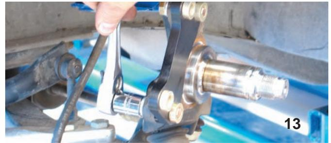
The Wilwood caliper bracket was connected to the spindle assembly and it was tightened in order to check the caliper to rotor centering. The caliper bolts were coated with Loctite and they were tightened to 75 ft-lbs using a foot-pound torque wrench.
