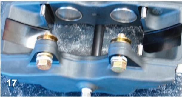
The caliper was bolted to the caliper bracket with two 1 ½-inch long 7/16-20 bolts. The bolt should be outfitted with a 0.063-inch washer on the outside of the caliper and in this case two 0.016-inch thick shims between the caliper and bracket. The shims are used to center the caliper over the rotor so the total number of shims used may change.
