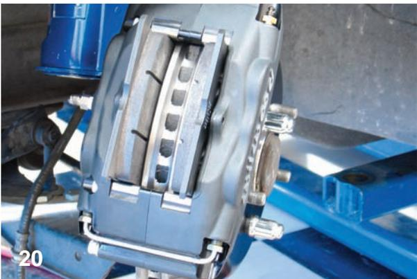
The caliper bridge bolt was removed and the BP-10 Smart Pads were installed.
