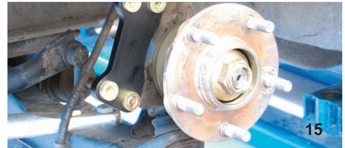
The hub was reinstalled on the spindle and tightened properly. This spindle bolt is a special locknut.
