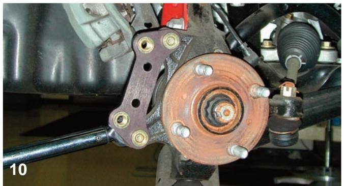
After the caliper mounting bolts were secured, the bolts were coated with Loctite 271 and then they were tightened to 75 ft-lbs.
