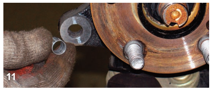
11 The original caliper mounting holes are slightly larger than the bolt size being used to secure the caliper brackets so the holes were filled with sleeves to make up the difference.
