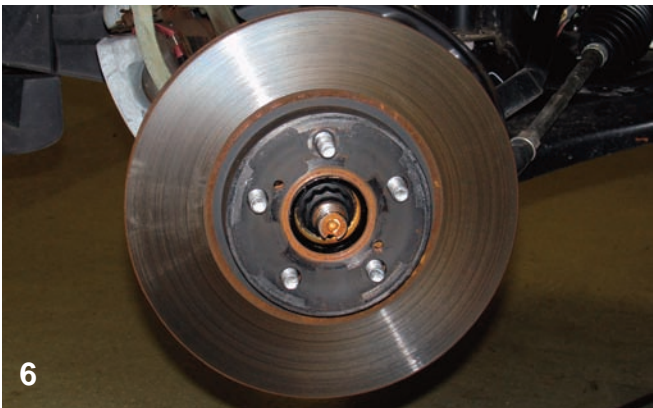
6 Here is the rotor after the caliper was removed. The rotor rides on the centering ring and it is held in place with the lug studs. Some persuasion may be needed to break the rotor away from the hub assembly.
