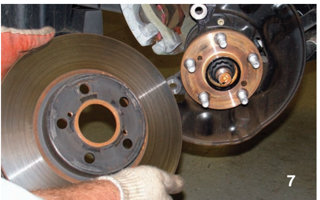
7 Here is the rotor after it was removed from the Hub assembly.
