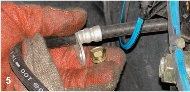
5 Here is the hose and the built-in bracket. It would be a good idea to fabricate a small bracket for the Wilwood Engineering 120-8336 hose so you should keep the bolt and reuse it.
