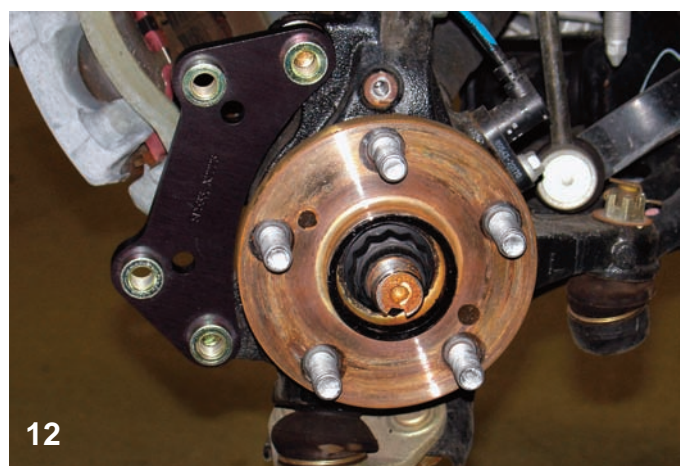
12 Here is the caliper bracket after it was connected to the original caliper mounting ears using the bolts and washers in the kit.. After the rotor to caliper centering is complete, the bolts should be coated with Loctite 271 and then the bolts should be tightened to 75 ft-lb.
