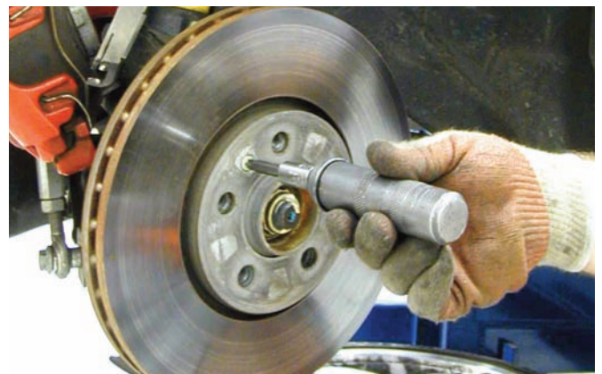
The rotor is connected to the hub assembly with a small screw. This screw was loosened with an impact screwdriver and then was removed as seen here. The same screw will be used to connect the Wilwood rotor.
