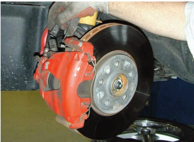
Before the caliper was removed, there was a small electrical plug that had to be disconnected.
