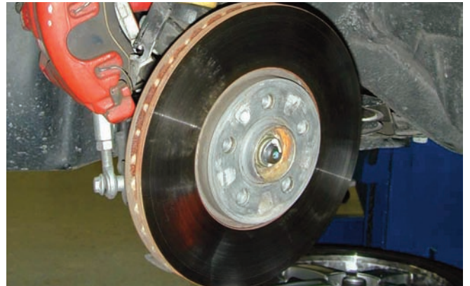
The caliper was removed and for now it was moved out of the way until the brake line could be removed and replaced.
