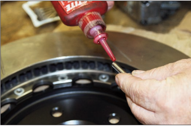
Sequence 7: Apply red Loctite ® 271 to the mounting bolts and thread into the hat.
