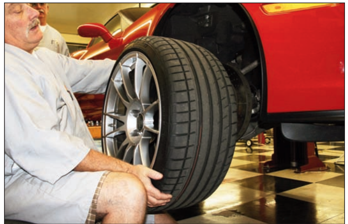
Sequence 12: Install the wheel and torque the lug nuts to manufacturer's specification. Rotate the wheel and check for any interference. Bed in the brake pads and rotor in a safe location before general use driving.
