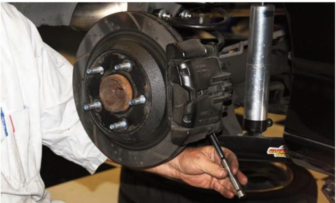
After the bolts were loose, they were disconnected using a small socket wrench. When the bolts were disconnected the caliper was removed.
