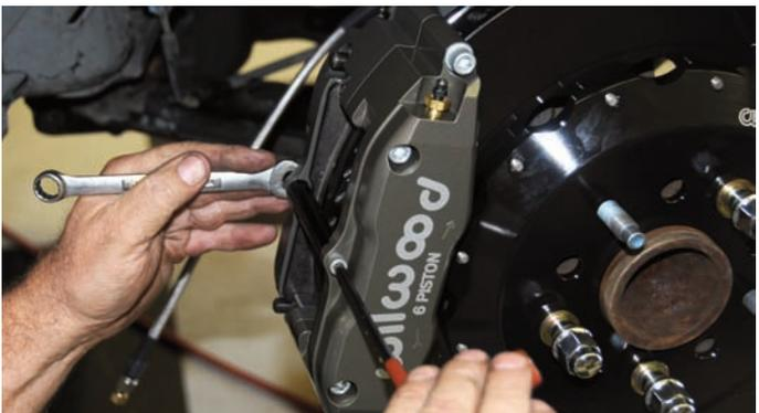
After the brake pads are in place, the bridge bolt was installed and it was tightened with an Allen wrench and an open-end wrench.
