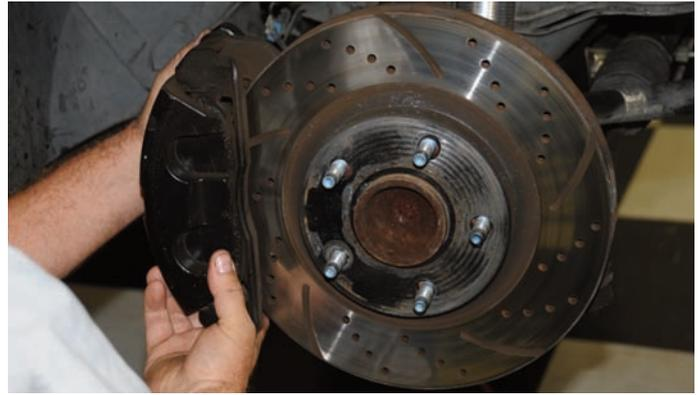
After the bolts were disconnected, the calipers were removed from the rotor assembly. This car is equipped with heavy cast iron calipers.
