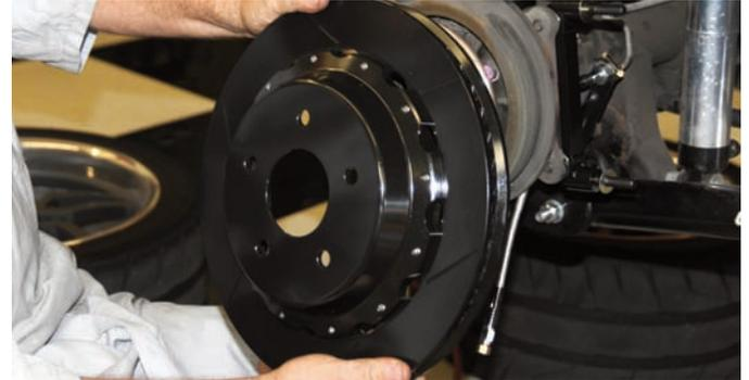
The rear rotor was assembled in the same manner as the front rotor. After it was assembled it was mounted on the rear hub assembly. This hub adapter works perfectly with the Camaro internal drum parking brake assembly.
