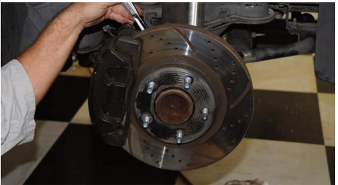
After the bolts were broken loose, they were removed quickly with a socket wrench. The drilled and slotted rotors on this car are not stock, they were upgraded in the past.
