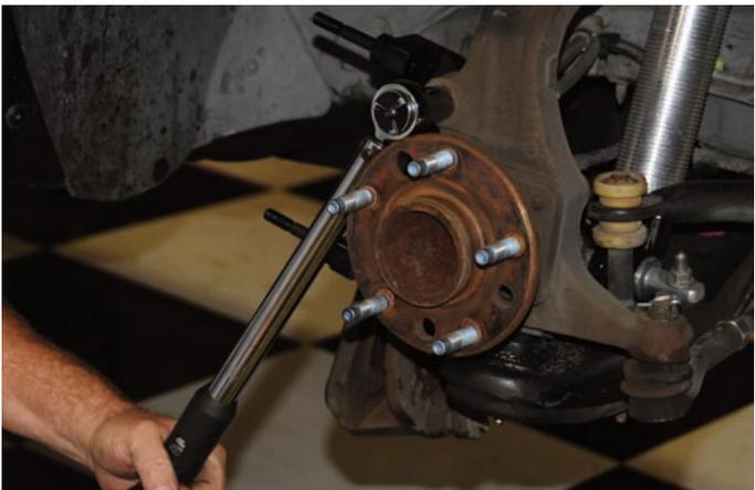
After the bracket is secure, the bolts should be tightened to 65 ft-lbs using a foot-pound torque wrench.
