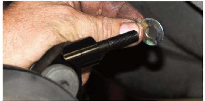
The caliper mounting bracket studs were loaded with a shim washer before the caliper was installed.
