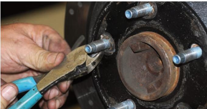
The small spinner ring was removed using cutting pliers. This rotor was connected with several small spinner nuts.
