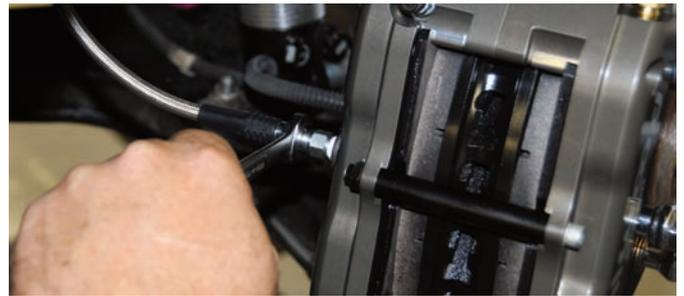
The Wilwood braided steel flex line was connected to the caliper inlet fitting. The aircraft-style line was super tight to make sure the connection was leak free.
