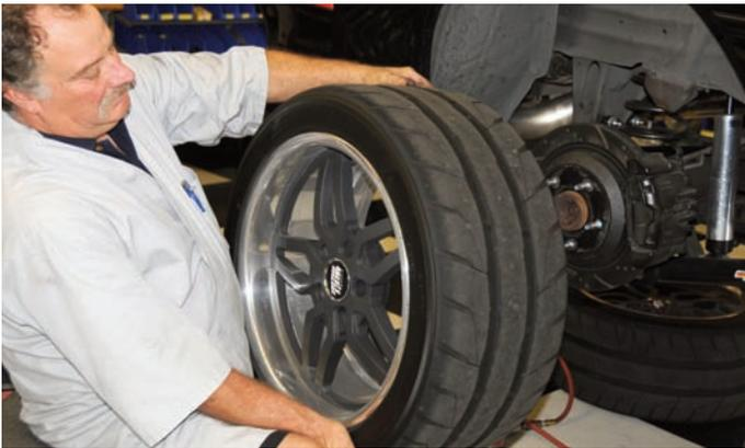
After the lug nuts have been removed the rear wheel and tire assembly could be lifted away from the car.
