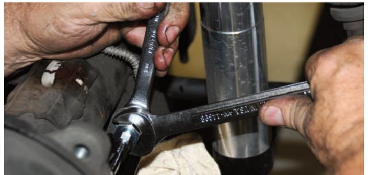
The Wilwood part number 220-9882 brake line was connected to the original steel line using the adapter fitting in the kit. After the hose was in place, it was secured to the bracket with a small spring clip.
