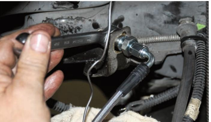
The Wilwood part number 220-6746 flex line was connected to the steel line using the adapter supplied in the kit. After the line was in place, the spring clip was installed to hold it to the bracket.
