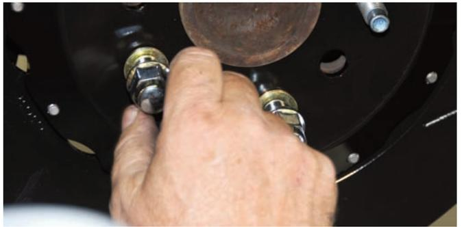
The rotor was connected to the hub assembly using three lug nuts. This will allow Tony to check the rotor to caliper centering to make sure it was the same as the other side.
