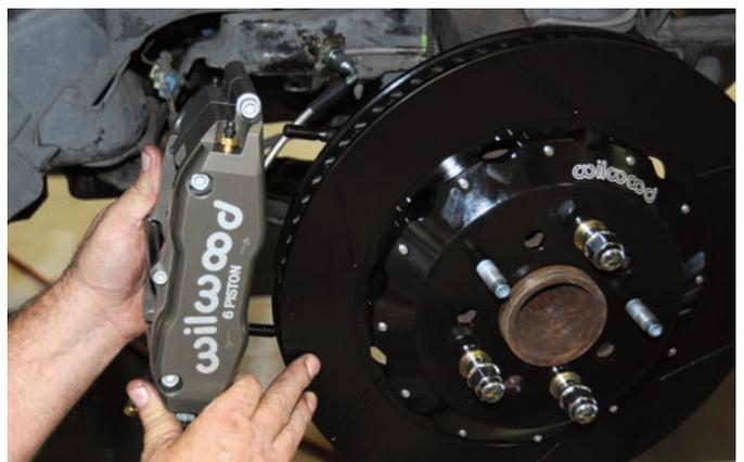
The caliper was placed over the studs and then it was lowered into place. This is a good time to check the caliper to rotor centering.
