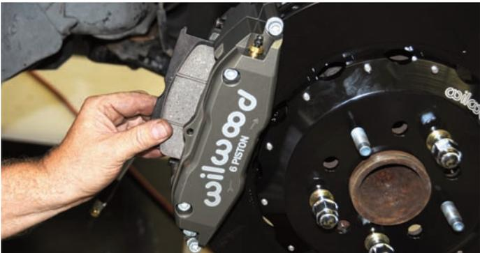
The bridge bolt was removed so that the BP-10 Smart Pads could be installed. Notice the arrow on the caliper indicating the direction the rotor will be moving in. There is a right and left side caliper, so make sure they are installed properly.
