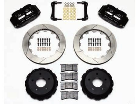
The Internal Drum Parking Brake Kit features Platinum-E coated Billet Narrow Superlite four-piston calipers, 12.90-inch E-coated slotted rotors, aluminum internal drum rotor adapters, caliper brackets, BP-10 Smart Pads, and all of the hardware required to finish the installation.
