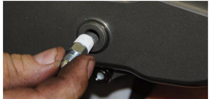
The caliper inlet fitting threads were coated with Teflon tape and then it was screwed into the caliper.
