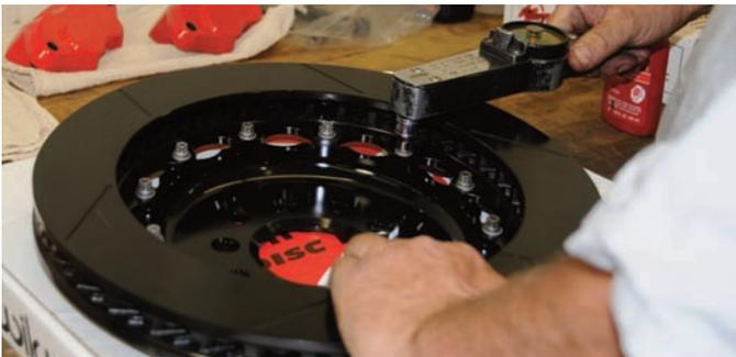
After the rotor adapter bolts were snug, they were tightened to 85 in-lbs using an inch pound torque wrench.
