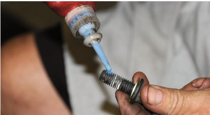
The original caliper mounting bolts were reused along with a new washer. The bolts were coated with Loctite 271 before the caliper brackets were installed.
