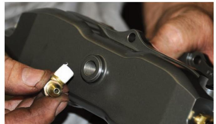
The rear caliper uses a 90-degree angle inlet fitting as seen here. The threads were covered with Teflon tape and then the fitting was screwed into the caliper.
