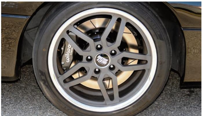
Here you can see the brake assembly through the spokes in the Camaro custom wheels. Notice that the pad bedding procedure cleaned the black coating off of the rotor face.
