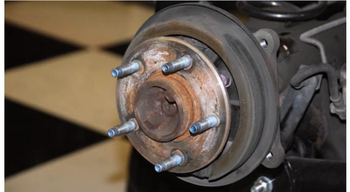
The Camaro uses a small drum-style parking brake assembly. The Wilwood rotor adapter was designed to work with this parking brake mechanism.
