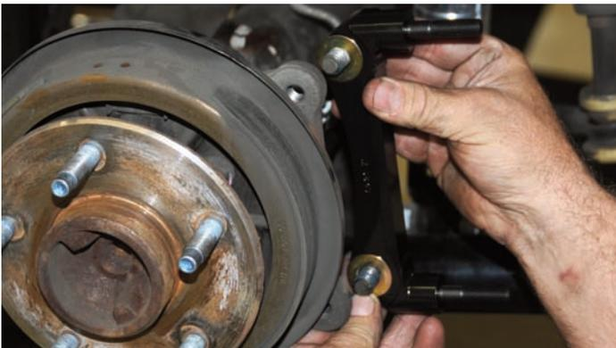
The caliper mounting brackets were installed to the original mounting ears. Notice the shim washer that is used between the bracket and the mounting ears.
