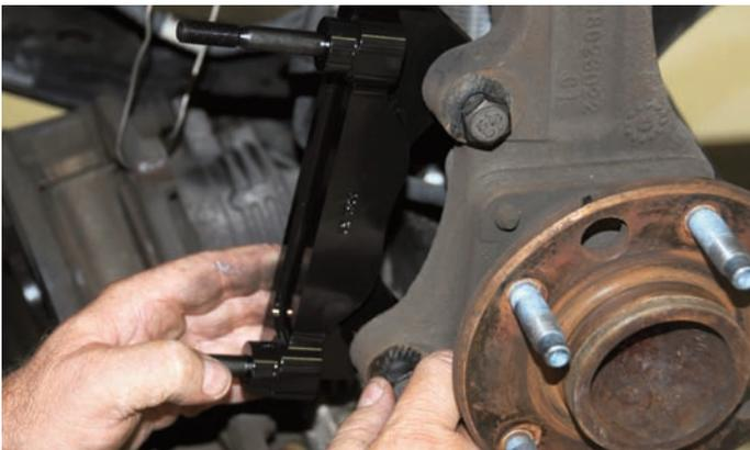
The bracket was set in place and then the bolts were connected to the bracket finger tight to start the process. After the bolts were connected they were tightened with a socket wrench.
