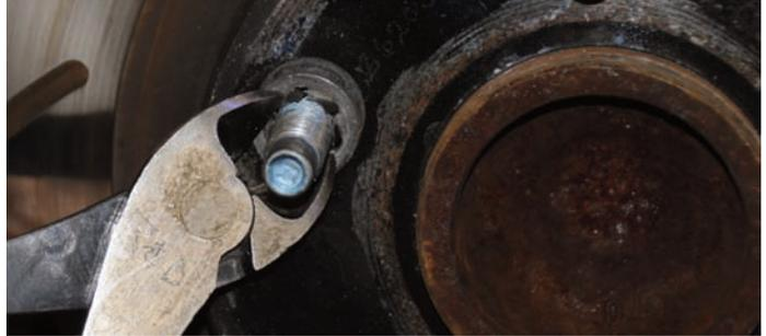
The rotor is connected to the caliper with these small spinner fasteners. The fasteners can be loosened a little but they usually break when pressure is applied.
