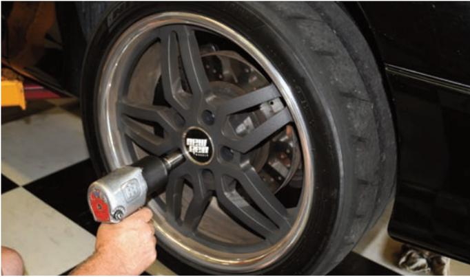
The Camaro was elevated to a comfortable working height and then the lug nuts were loosened with an Impact Gun.
