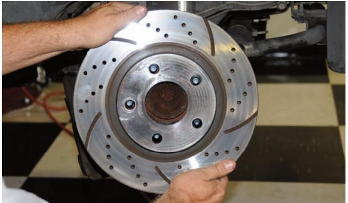
The aftermarket drilled and slotted rotor was removed from the hub assembly and it was set aside.
