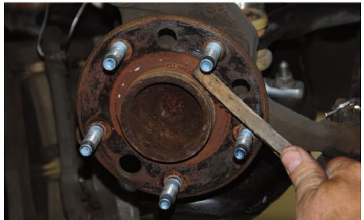
After the rotor was removed, the hub assembly was cleaned thoroughly with a wire brush.
