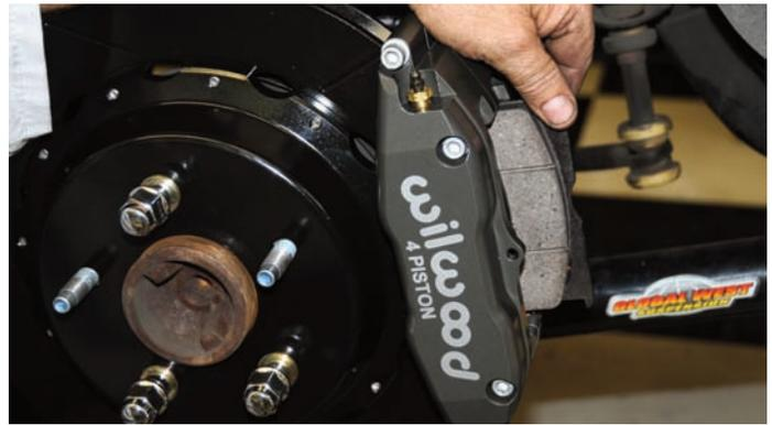
The bridge bolt was removed so that the BP-10 Smart Pads could be installed.
