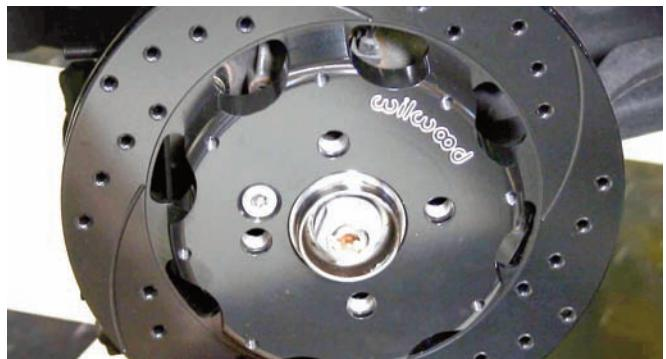
The rotor was installed on the hub assembly and the holes were aligned so that the mounting bolt could be installed and tightened.
