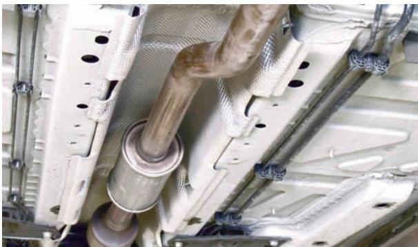
In order to complete the parking brake line routing, the bolts were removed from the second from rear heat shield and then it was removed.
