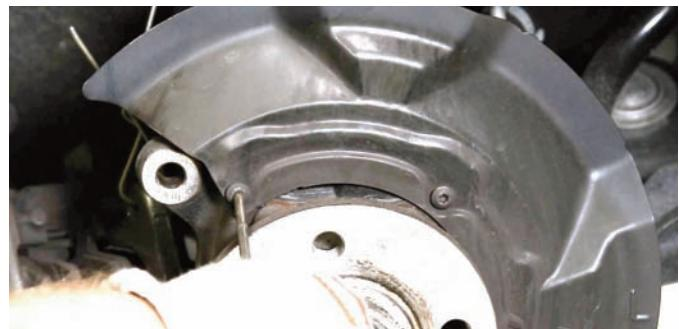
Using a torx screwdriver, the small screws that fasten the dust shield to the hub assembly were removed.
