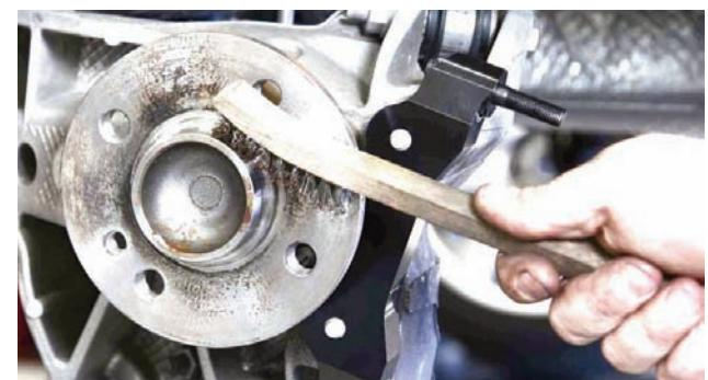
Grease, dirt or debris of any kind was removed from the face of the hub assembly, especially around the centering ring.
