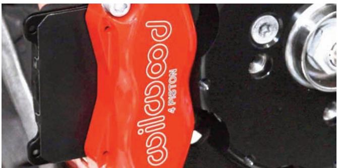
After the caliper was centered, the pads were installed from the top of the caliper. The pads were fastened with the Quick-clip pad retainer.
