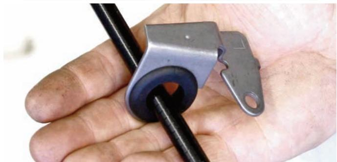
The mounting brackets that were previously removed were modified so the new lines could be run through. Using two grommets, they were placed over the line and were pressed into the small brackets as seen here. After the lines were in place, the small brackets were bolted back on the control arms.
