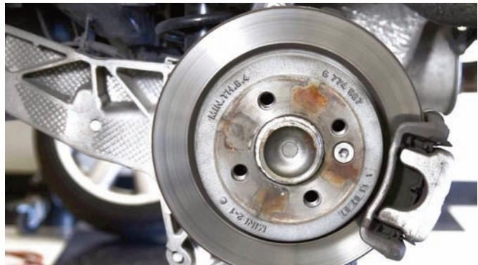
Here is a look at the factory disc brake setup that connects to a hub assembly that rides on a large aluminum lower control arm.
