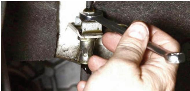
The old brake hose was removed and the new Wilwood part number 220-8491 was installed remembering to install the rubber grommet that were removed from the original hose. The hole in the bracket will have to be enlarged to hold the fitting used to adapt the Wilwood Flexline to the original steel line.
