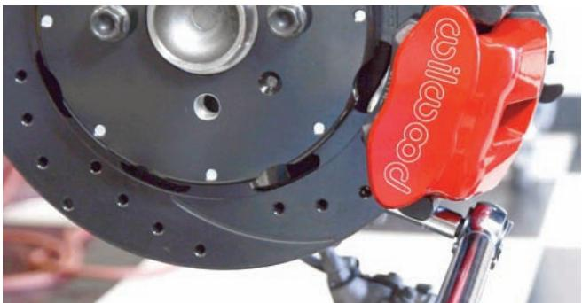
The caliper was attached to the bracket and then the caliper to rotor centering was examined. Adding or subtracting shims can be used for adjustments. After the rotor is centered in the caliper, the bolts were tightened to 30 ft-lbs using a torque wrench.
