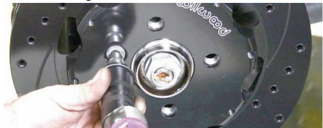
The rotor was attached to the hub assembly using the same torx bolt that fastened the original rotor. The impact screwdriver is reversible so a few whacks of the hammer got the bolt very tight.
