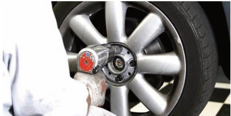
Using a floor jack, the front of the Mini was raised and was placed on jack stands. The hubcaps were removed to access the lug bolts. Using the proper size socket and an impact gun the lug bolts were disconnected and the wheels and tires were removed.
