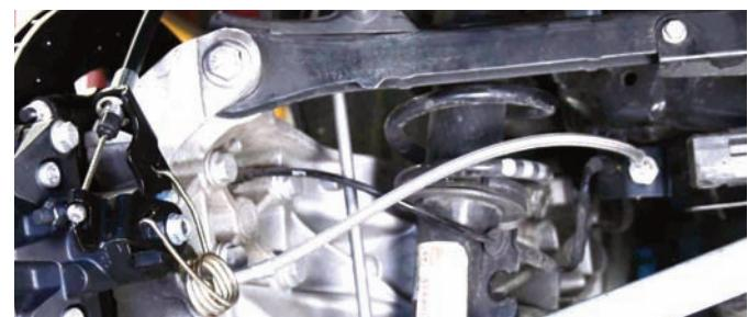
Here is the Wilwood part number 220-10879 braided steel Flexline running from the caliper to the bracket holding the steel line and adapter fitting. The line was routed away from any moving parts.
