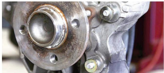
The caliper bracket bolts to the same location the original caliper bolted to. Here you can see the bolts in the holes and they will be used with a two shims per bolt.
