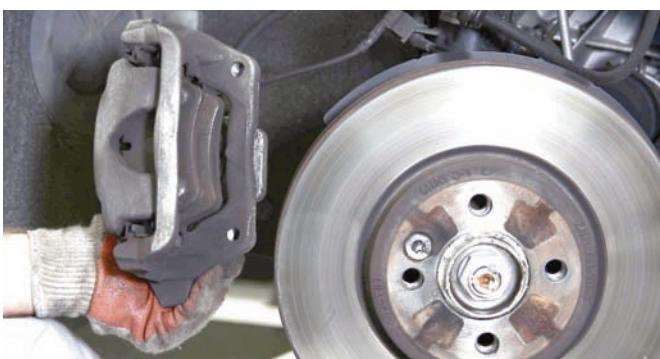
After the bolts were disconnected, the cast iron caliper was removed from the brake assembly. The new brake caliper is much lighter than the old caliper.
