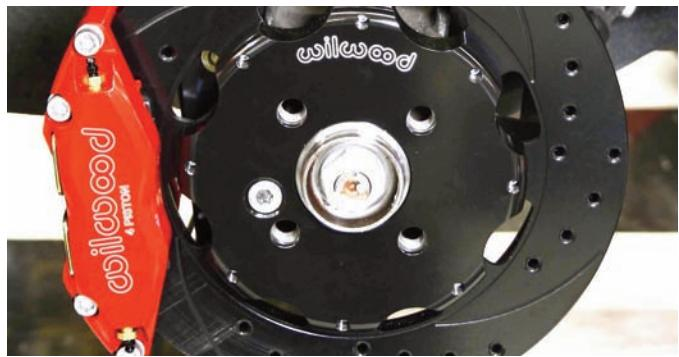
The finished brake assembly is looking good with the bright red caliper and black E-coated rotor. This system will improve the Mini braking, plus it looks nice doing it.
