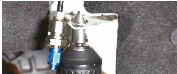
After the original line was removed the bracket was drilled out just a little so that the adapter fitting seen here can be installed in the bracket.
