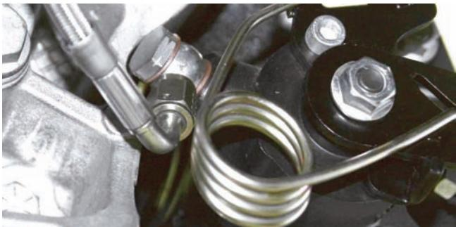
The protective rubber plug was removed from the caliper inlet. The banjo fitting was installed making sure there was Teflon tape on the banjo nut. The Wilwood part number 220-10879 was connected to the fitting and then the line was routed toward the steel line bracket.
