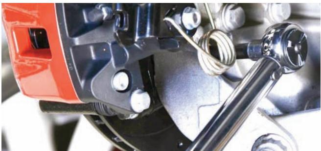
The bolts for the caliper mounting bracket were coated with Loctite 271 and then they were tightened to 22 ft-lbs.
