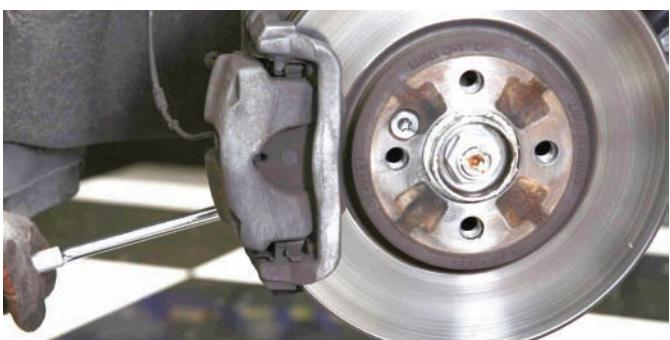
Using a breaker bar and the correct size socket, the caliper bolts were disconnected from the front hub assembly.
