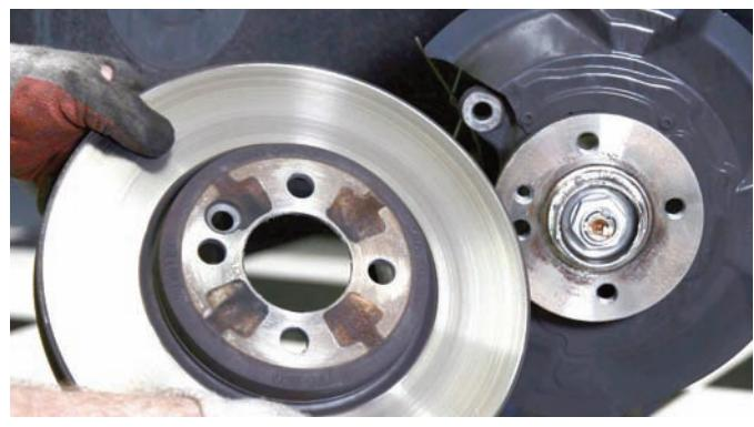
The rotor was tapped with a rubber mallet on the back-side to break it loose from the hub assembly. When it was loose, it was removed from the assembly.
