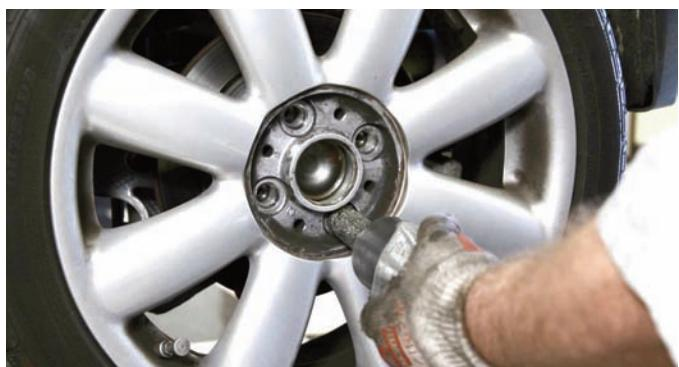
The rear of the Mini was raised and the jack stands were placed under the car for safety. The hubcaps were removed and then the lug bolts were disconnected with the correct size socket on an impact gun.
