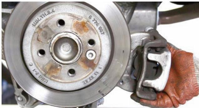
After the bolts were disconnected, the caliper was removed from the bracket and the car.
