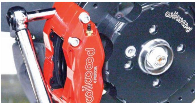
The caliper was placed on the caliper bracket and then the washers and locknuts were installed. Make sure the rotor is centered in the caliper, and when it is, the studs were lightly oiled and the mounting nuts were tightened to 30 ft-lbs using a torque wrench.
