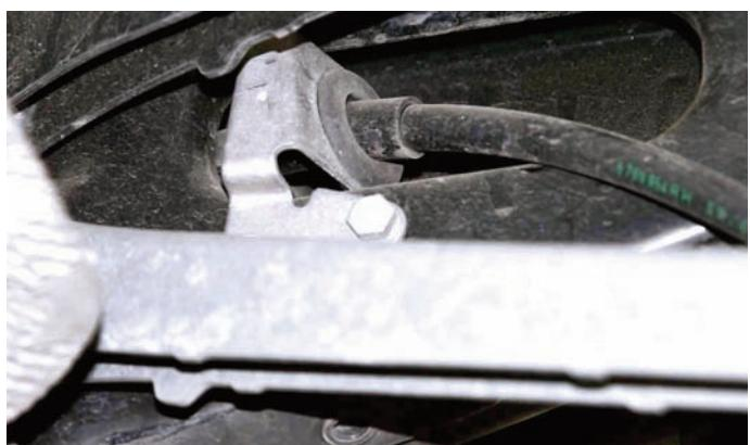
Here is the bracket after it was bolted in place. The brackets keep the parking brake lines safe and out of the way of any moving parts.
