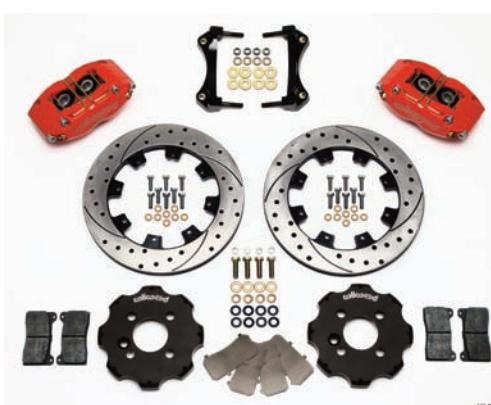
The Wilwood part number 140-8528 front disc brake kit comes complete with the rotors, hats, DynaPro calipers, pads, caliper brackets and all of the hardware required to finish the installation. The kit ordered features red calipers and the slotted and cross-drilled rotors.
