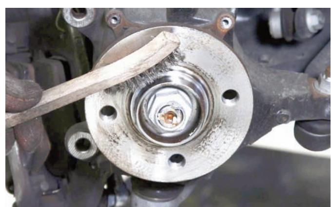
Before going any further, a wire brush was used to clean the grease and grime away from the hub locator on the hub.
