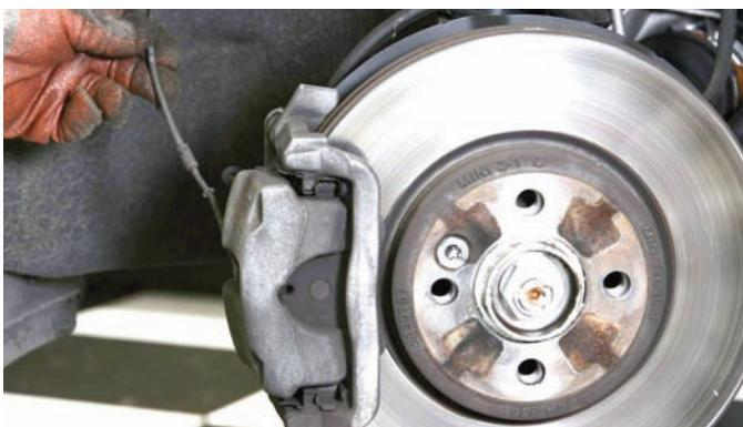
The original flexible brake line was disconnected from the steel hard line in preparation of removing the caliper. There is a rubber grommet on each flex line so it was removed and retained for reinstallation on the new Wilwood Flexline.
