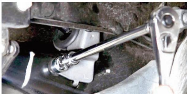
The bolts fastening the cable brackets on the rear suspension arms were also removed so they can be slightly modified.
