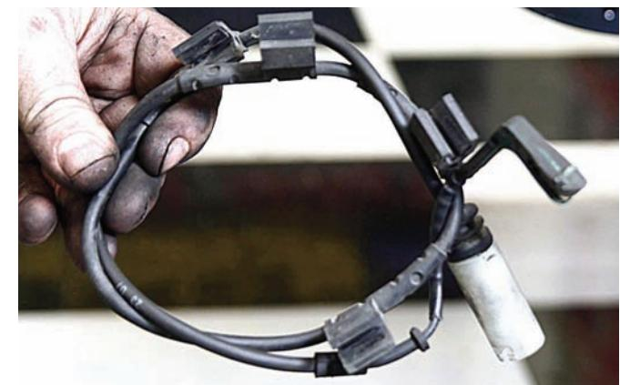
The brake wear sensor line was wrapped up and it can be installed in an inconspicuous place while connected in the car. If the brake sensor line is removed completely, the brake wear dash warning light will remain on.
