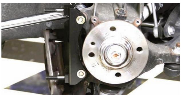
The bracket should be tight to check the rotor to caliper centering. It should be centered but if it is not, shims can be added or subtracted to get it perfect. After the centering was perfect the bracket bolts were coated with Loctite 271 and then they were tightened to 75 ft-lbs.
