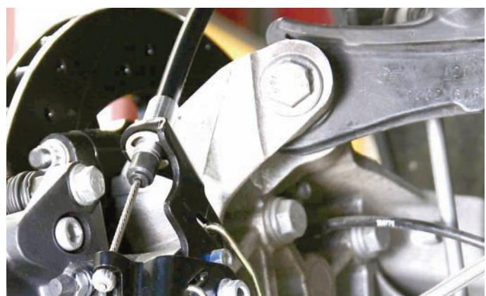
The lines were run forward and here is how they were attached to the master cylinder lever.
