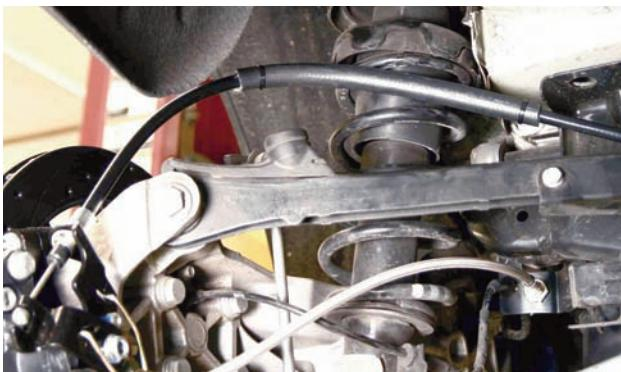
The parking brake line was wrapped with a rubber hose for added protection. It is secured to the line with a pair of black tie wraps.
