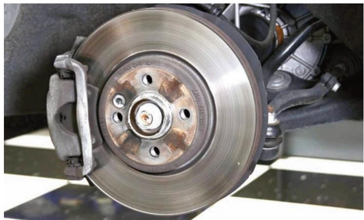
After the wheels and tires were removed, you can see the original Mini brakes and rotors. This car uses lug bolts instead of lug nuts and the rotor is secured to the hub with a large torx bolt.
