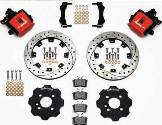
The Wilwood part number 140-10885 rear disc brake kit comes complete with the rotors, hats, Combination Parking Brake (CPB) calipers, pads, caliper brackets and all of the hardware required to finish the installation. The kit ordered features red calipers and cross-drilled rotors.
