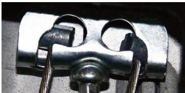
The console was removed to access the hand-brake cable equalizer with two cables going toward the rear. The two cables were removed from the equalizer and they were pushed toward the rear. The OEM cable end clips are hidden at the very rear of the tunnel and hidden under the rearward brace. Using a four-inch long metal tube, it was forcefully placed into each clip and then the cable was twisted and pulled out of the holes.
