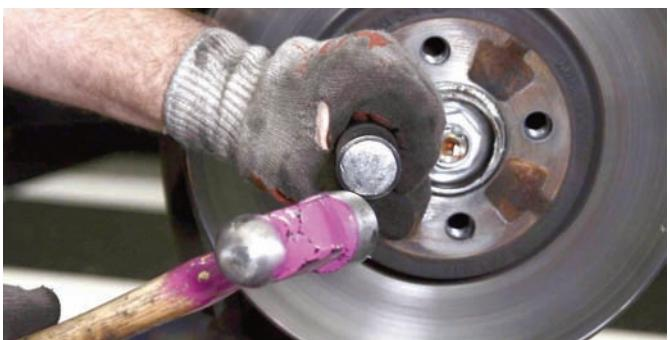
The torx bolt that secures the rotor to the hub was very tight, so it was loosened with an impact screwdriver. The bolts were retained because they will be used to fasten the new rotors.
