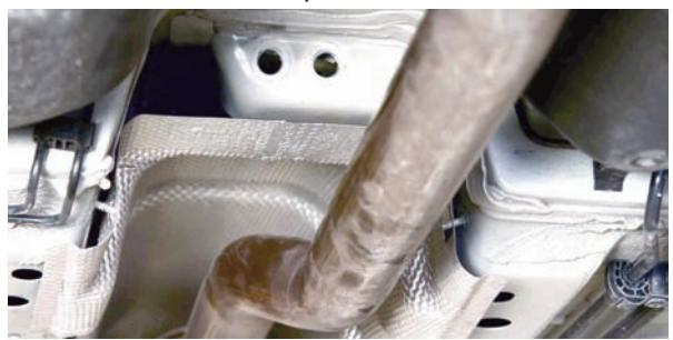
The two holes seen at the top of the photo were enlarged to 0.530-inch. The new cables were slid into the enlarged holes and were pressed into place in the equalizer.
