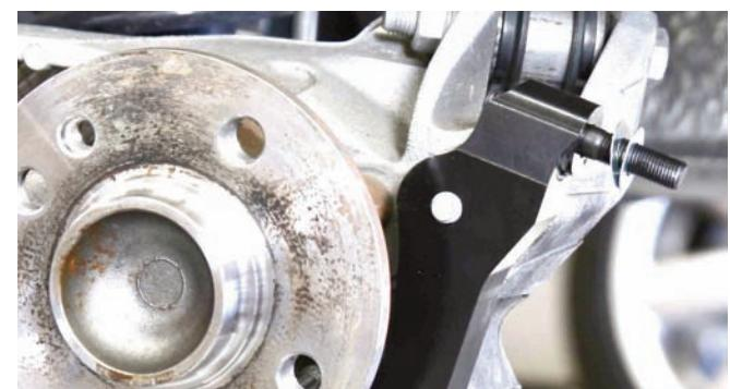
Before the caliper was installed, the bracket studs were loaded with two shims per stud.
