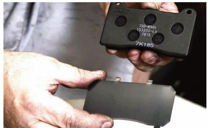
The adhesive backing was removed from the anti-squeal plate and then it was attached to the rear side of the brake pad. The tabs were bent over the pad baking plate to keep them in place.
