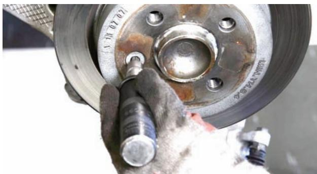
The torque bolt that secures the rotor to the hub assembly was removed with an impact screwdriver.
