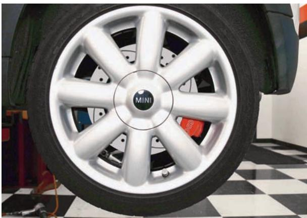
The wheel was installed and the Mini was ready to have the brakes bled followed by the brake bedding process. When that was finished, the Mini brakes were working terrific and they also look attractive behind the Mini wheel spokes
