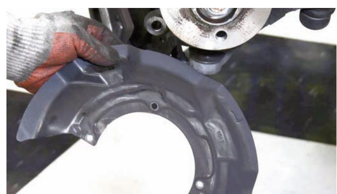
The dust shields were discarded because they will not be used with the new brakes.
