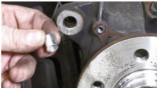
The original caliper mounting holes are rather large, so bushings are used in the top and bottom hole to downsize the holes.
