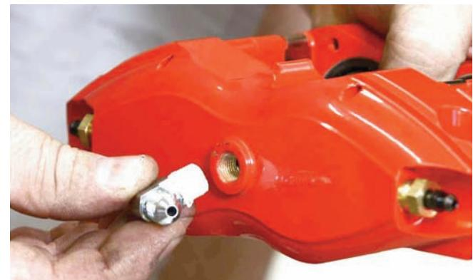
The inlet fitting was coated with Teflon tape and then it was screwed into the caliper. The fitting should be pointing upward.
