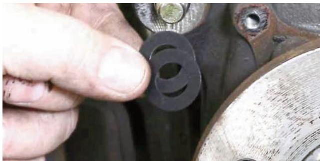
The bolts were installed into the original caliper mounting holes and two shims were installed.
