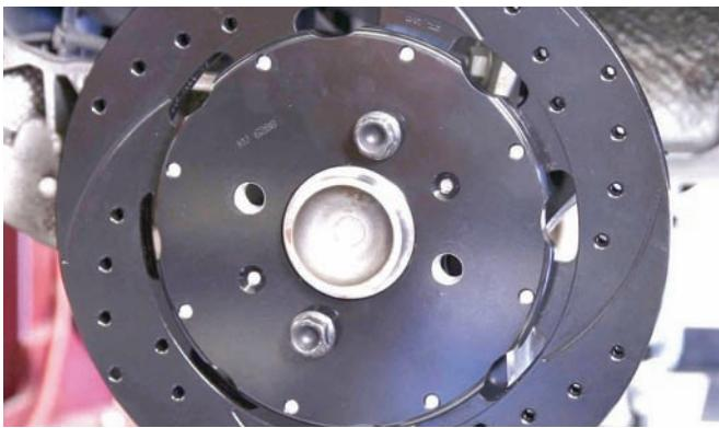
The rotor was placed on the hub assembly and then it was tightened with two lug bolts.
