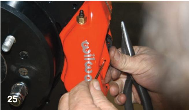
After the pads were in place, the long cotter key was installed to secure them.
