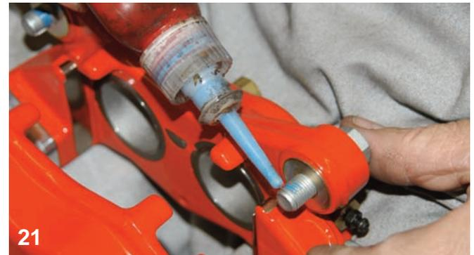
It was determined that only one shim washer was required to center the caliper and rotor. Here the attachment bolt was being coated with Loctite prior to installing the caliper.
