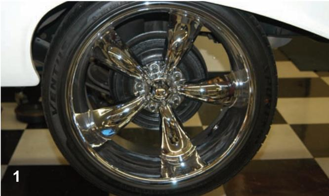
Here is the '61 Chevy with the large 20-inch five spoke rear wheels. The open spokes in the wheels clearly show the little rear drum brakes. In this Chevy's case the brake installation will not only be a performance improvement, it will also be an appearance enhancement.
