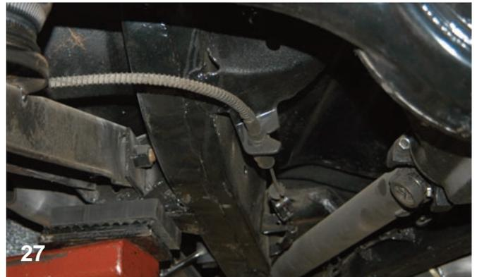
The original emergency brake cable will no longer be used. The cable has to be released and the cable has to be removed from the frame bracket.
