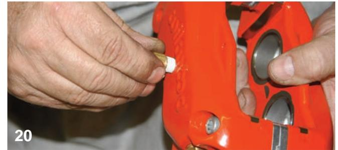
The inlet fitting threads were covered with PTFE Thread Tape and then the fitting was screwed into the caliper.
