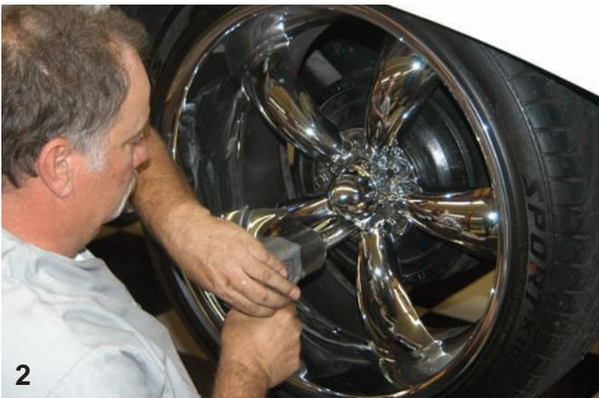
The Chevy was safely elevated so that the wheels and tires could be removed. Using an impact gun and the appropriate size socket, the lug nuts were disconnected from the attractive five-spoke wheels.
