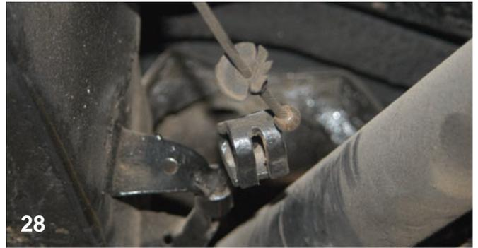
Here is the rear cable after it was disconnected from the main parking brake cable.
