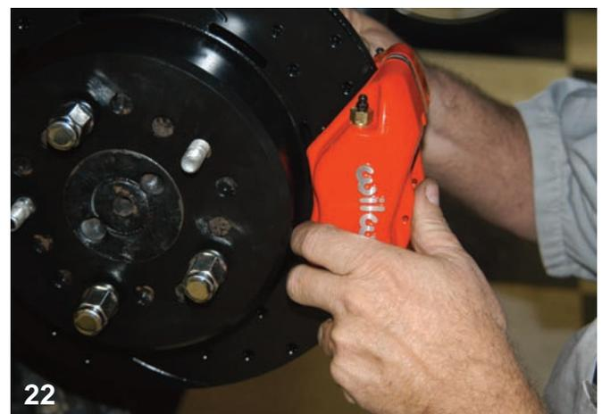
The caliper was placed over the rotor and the connections were aligned with the bracket holes. The bolts were connected finger tight to start with.
