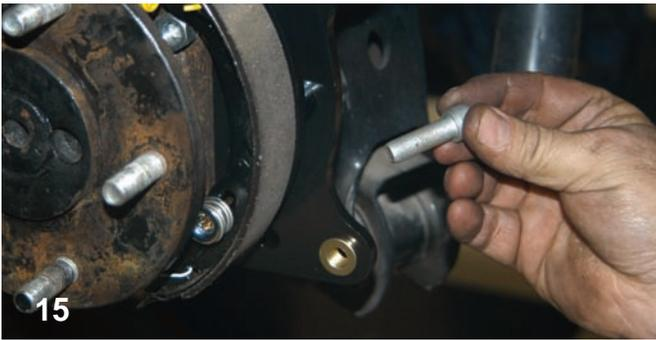
Four of these bolts will be used to install the parking brake mechanism and bearing retainer plate to the axle flange. The bolts are installed from the backside of the axle flange as shown here.
