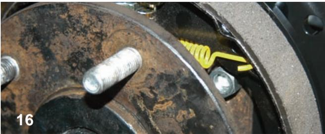
Peeking through the opening, you can see the nut on the bolt. Before the nut was installed, a small flat washer was placed on the bolt. This is a tough area to reach, so you will have to be tricky to get the nut connected to the bolt. Tony used a magnet tool to get the parts started.
