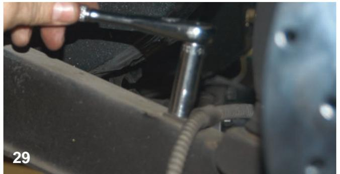
The parking brake cable bracket is attached to the axle strut with a small bolt. Here the bolt is being removed. The small bracket can be used to secure the new cable that will be installed.
