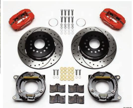
The '59-'62 Chevy rear brake kit features Dynalite calipers, rear internal drum brake units with built-in caliper brackets, rotors that work with the internal drum brake mechanism, BP-10 Smart Pads and all of the hardware required to finish the installation. The standard kit number is 140-11828 but with the red calipers and drilled and slotted rotors the number is 140-11828-DR.
