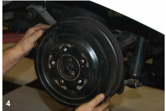
The brake drum was moved side-to-side to release it from the centering ring. After it was loose, it was removed from the car.
