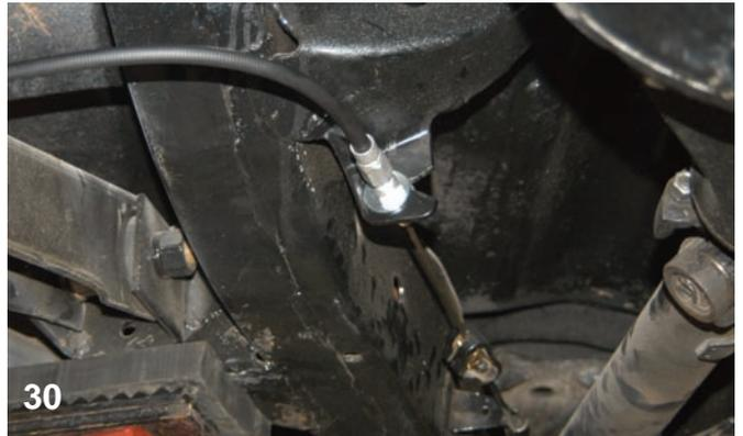
Using a Wilwood universal brake cable kit, a new brake cable mechanism was installed.
