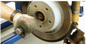
Using an impact screwdriver, the screws that secure the rotor to the hub assembly were removed.
