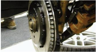
The caliper mounting bracket was held against the original mounting ears and then the bolts and washers were connected. Under the head the original washer was used and between the caliper and mounting ears a flat washer was used.
