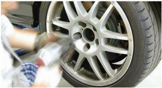
The front of the BMW was raised up using a floor jack and then jack stands were placed underneath it to keep it elevated. Using an impact gun and the correct size socket, the lug bolts were disconnected so the wheels and tires could be removed.
