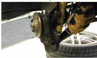
After the rotor was removed, you can see the mounting ears that the caliper bracket will bolt onto.
