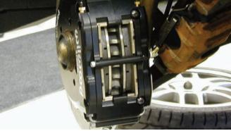
After the caliper was secure and the brake pads were seated, the bridge bolt was connected to keep the pads in place.
