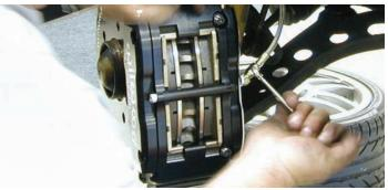
The Wilwood 220-8799 brake hose was connected to the inlet connection in the Caliper using a line wrench.
