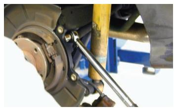
The caliper mounting bolts were coated with Loctite 271 and then they were tightened to 30 ft-lbs using a footpound torque wrench.
