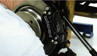
After the caliper is centered over the rotor, the mounting bolts were coated with Loctite 271 and then they were tightened to 30 ft-lbs.
