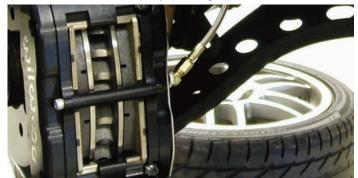
Here is a closer look at the braided steel hose connection and the direction of the inlet fitting. You can wrap Teflon tape on the fitting and make sure the aircraft style fitting is tight to avoid any leaks.
