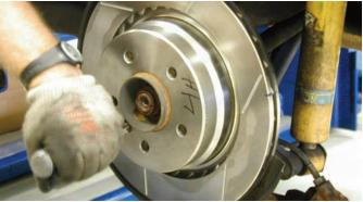
The rotor was placed on the hub assembly and then the original screw was used to secure it. Some parking brake shoe adjustments may be needed to get the shoes close to the hub assembly.
