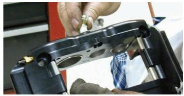
The fluid inlet fitting threads were wrapped with Teflon tape and then the fitting was screwed into the side of the caliper.
