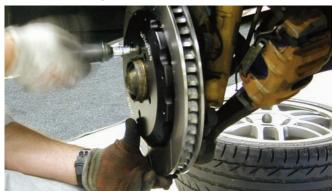
The rotor was connected to the hat assembly using the bolts and washers in the kit. The bolts were coated with Loctite 271 and then they were tightened in an alternating sequence to 85 in-lbs. After the rotor was assembled it was placed on the hub mounting flange and it was connected with the original screws.
