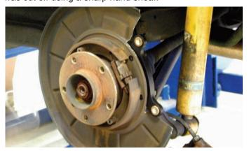
Here is the dust shield after the material was removed. This should allow enough clearance for the new caliper.
