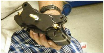
The caliper inlet fitting was covered with Teflon tape and then the fitting was screwed into the caliper.
