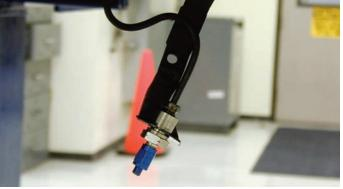
The rear hose bracket was modified to accept the adapter fitting. The bracket was reinstalled in the car and the Wilwood 220-8799 hose kit was installed following the methods used on the front hoses.
