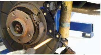
The caliper bracket was connected to the mounting ears to determine where the dust shield will have to be cut to allow the use of a larger rear caliper.
