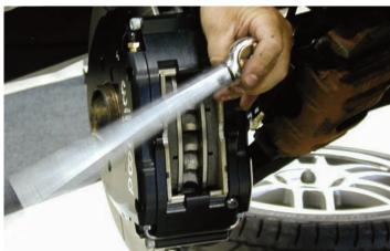
The mounting washers and locknuts were connected to the studs and then the nuts were tightened to 35 ft-lbs using a foot-pound torque wrench.
