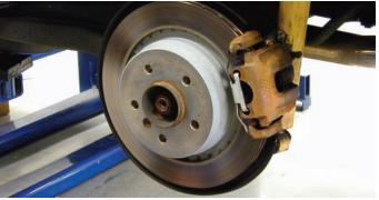
The front of the car was lowered and the rear was raised up to access the rear brakes. The wheels and tires were removed to reveal the original rear brake system.
