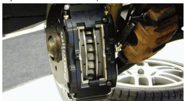
Here you can see that the rotor is centered in the caliper and the radius of the brake pads matches the radius of the rotor.
