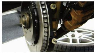
Before the caliper was installed, flat washers were loaded on the mounting studs. These washers can be used to raise or lower the caliper.
