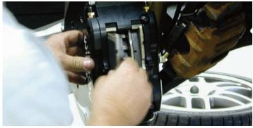
The caliper was placed on the mounting studs until it was fully seated and then the brake pads were installed.
