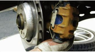
The two bolts that secure the original caliper to the mounting ears were disconnected. After they were removed, the caliper could be lifted off of the rotor.
