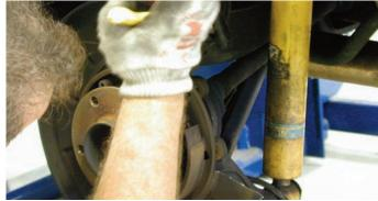
After the dust shield was marked, the area to be removed was cut off using a sharp hand shear.
