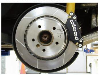
Here is the rear brake assembly finished and ready for action on the street or on the track. The four-piston rear brakes will work perfectly with the larger six-piston front brakes to provide perfect front to rear brake bias. Now the brake bleeding and pad bedding can begin.
