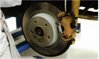
The two bolts that secure the caliper to the bracket were removed with a large breaker bar. After the bolts were disconnected the caliper was removed from the rotor.
