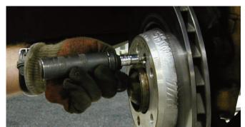
Using an impact screwdriver, the screws that secure the rotor to the hub assembly were disconnected.
