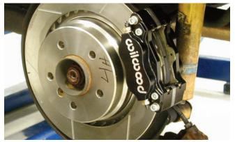
The caliper was connected to the bracket assembly using the screws and washers in the kit. The caliper to rotor centering should be checked and adjusted with shims if it is necessary.
