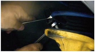
The original rubber caliper line was disconnected from the steel hard line using a line wrench.
