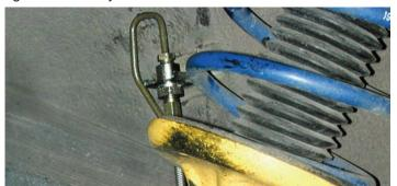
The steel line and adapter fitting were reinstalled in the frame bracket and the Wilwood line was connected. The original brake clip can be used to hold the line in place.
