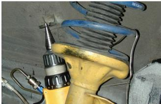
The hole in the original hose bracket was slightly under size for the adapter fitting so it was enlarged with a drill motor and a step drill.
