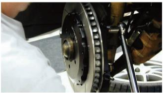
The caliper to rotor centering was checked and when it was determined that it was fine, the caliper bolts were coated with Loctite 271 and then they were tightened to 65 ft-lbs.
