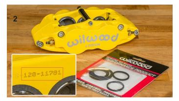
The caliper we are going to rebuild is a Forged Narrow Superlite 6R. We found the caliper part number stamped on the inside of the caliper, 120-11781, and cross-referenced it to the o-ring kit, 130-5972, on the Wilwood website or by contacting a Wilwood dealer.
