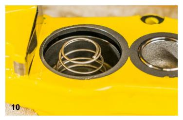
Using a clean towel lay the caliper on its side and center the spring inside the bore.
