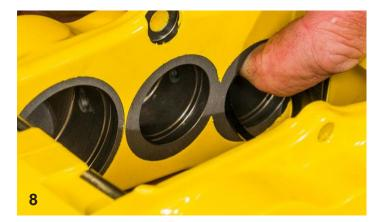
Insert the lubricated o-rings into the appropriate size bore and properly seat them into the seal gland making sure they are not twisted or pinched in any way. Test the seating by running your finger around the bore and make sure the seal is flat to the caliper bore.
