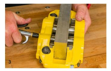
A block of aluminum, or wood, is used inside the caliper to limit the outward movement of the pistons when applying a little air pressure to the caliper inlet. DO NOT apply air without blocking the pistons as they can shoot out at a high velocity, and make sure your fingers are clear of the area.
