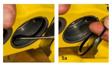
Using a small screwdriver or pick, remove the old o-rings from the piston bores. Do this carefully to prevent scratching the bores of the caliper body.
