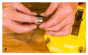
Using more DOT 3 or DOT 4 brake fluid from the lubrication tray, oil the outside and rear of the pistons.
