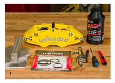
There is a square o-ring kit for every caliper Wilwood manufactures like this Forged Narrow Superlite 6R caliper. Tools to have on hand to make the job easier would be aluminum blocks (or wood), compressed air with blowgun nozzle, flathead screwdriver, razor knife, and Wilwood brake fluid.
