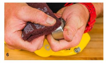
To prepare the pistons for reinstall, either very lightly clean them with a mild abrasive scratch pad, or use a clean, lint-free rag and some brake cleaner. Also, inspect the inside of the caliper bores to make sure they are in good condition – do not use any abrasives inside the caliper bores. Wipe them with brake cleaner on a clean lint-free rag.
