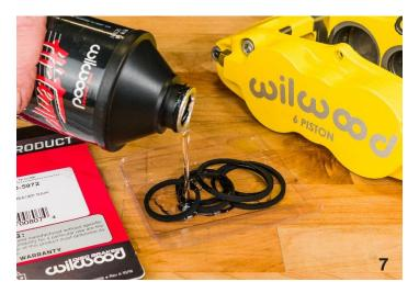
Use the plastic blister from the package as a tray and pour in some DOT 3 or DOT 4 fluid to lubricate the new o-rings sufficiently on all sides.
