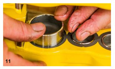
Slowly insert each piston and make sure you use plenty of lubrication, so they slide in easily without gripping or displacing the o-rings. Flip the caliper over and repeat steps from images 10 and 11 for the remaining pistons.
