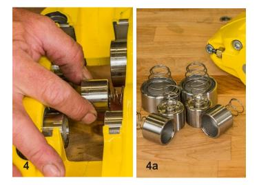
Carefully remove all the pistons and springs and set aside. Inspect the pistons, and if they are in good condition, they will be fine to use again during the rebuild.
