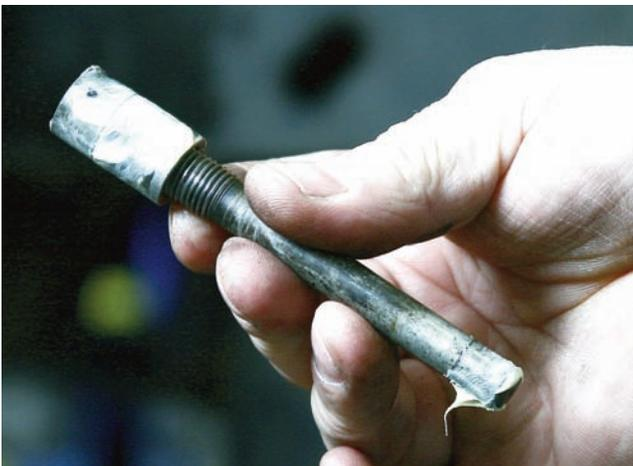
The sleeve was placed over the Wilwood mounting bolt and then they were coated with white grease before installation.
