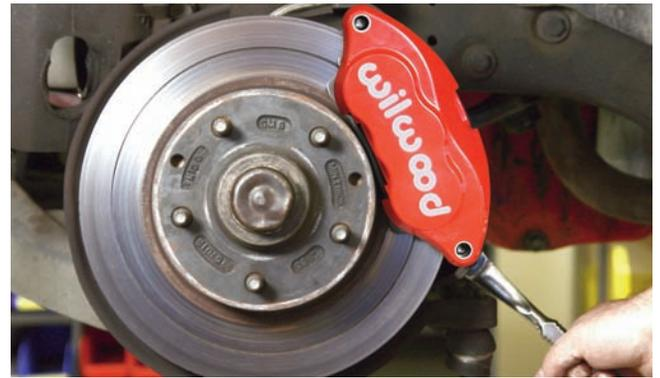
The Wilwood D52 caliper was installed by matching the mounting holes with the holes in the spindle bracket and then the two long Allen head slide bolts were installed. White grease should be applied to the slide portion of the bolts not the threads. At this point the banjo fitting can be installed making sure the threads are coated with Teflon tape. Also make sure the outside radius of the brake pad is aligned with the outside radius of the rotor face.
