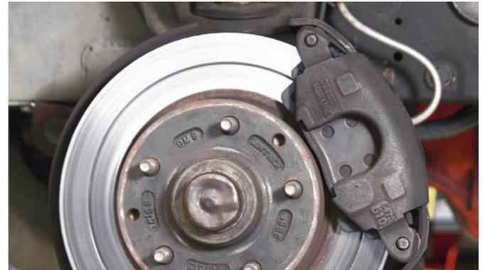
Here is the brake assembly after the tire and wheel were removed. Like we mentioned earlier, this would be the time to have the rotor surfaced if you find that it is necessary.
