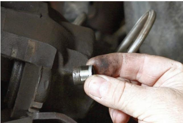
The old calipers were removed and here is the original sleeve. This one is worn out so it is a good idea to replace it with a new one.
