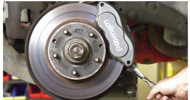
If you own an original muscle car and want to maintain a more original appearance you can upgrade the brake system by adding the gray (Platinum E) calipers, which are closer to the original color of the cast iron calipers. After the caliper is secured in place the flex line can be installed. You can use the original line but make sure you replace the copper crush washers. You can also upgrade the flex line by installing Wilwood part number 220-7056 lines to the banjo fittings and tighten.
