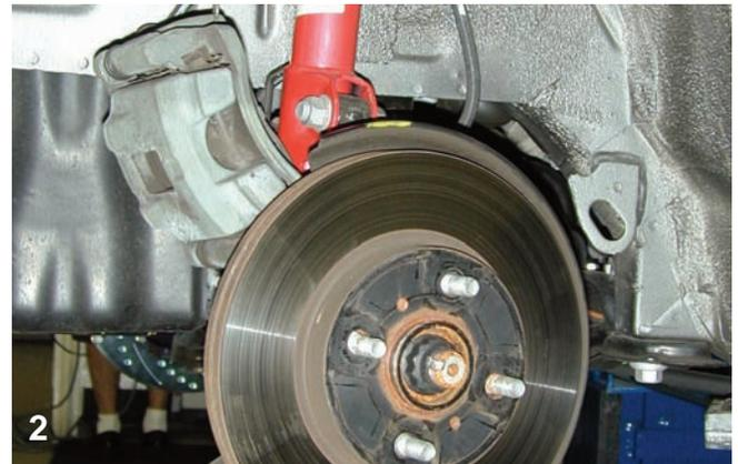
2 The two bolts that secure the caliper to the mounting ears were disconnected and then the caliper was removed from the assembly. The caliper was hung on a hook until the lines are changed over.
