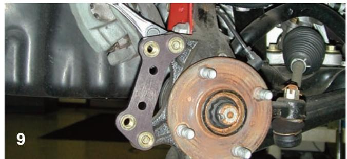
The caliper adapter was bolted to the ears using the bolts and washers in the kit.
