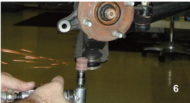
The lower ball joint on this particular car was very close to the rotor so it was necessary to give the rotor some additional clearance. The lower ball joint connection was trimmed just a little with a coarse grit barrel sander.
