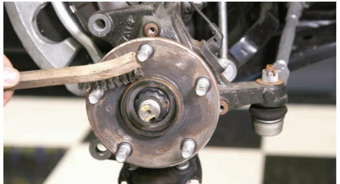
The hub assembly was thoroughly cleaned with a wire brush to remove any grease or debris.
