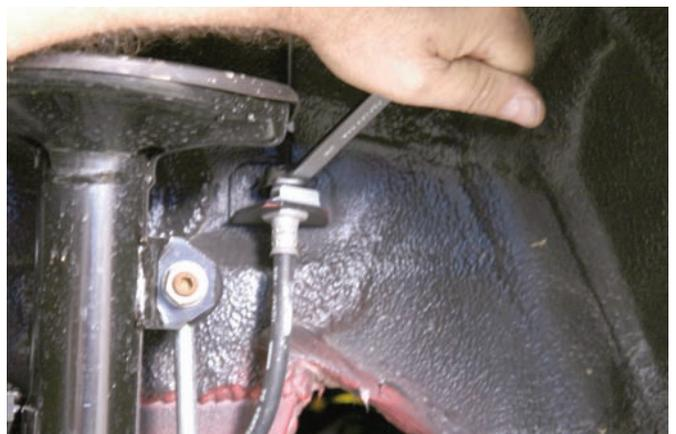
The rubber line was disconnected from the hard line using a line wrench. This connection is located on the inner fender well behind the strut.
