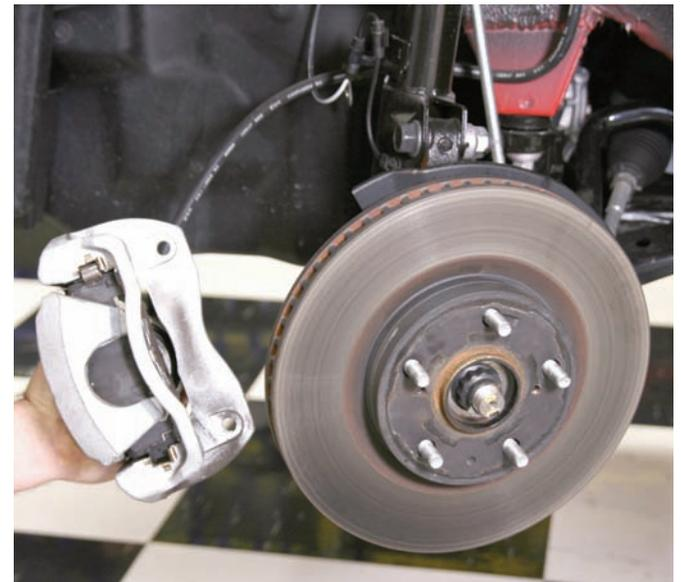
The caliper was removed from the assembly, but at this point it will remain hooked to the system.
