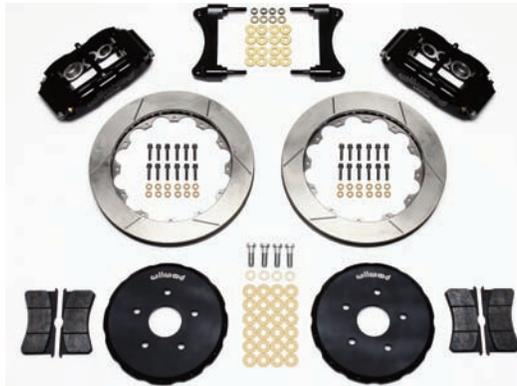
The toyota was outfitted with a Wilwood part number 140-10752 disc brake kit that features Superlite 6R calipers and slotted 12.90-inch rotors with aluminum rotor adapters. The kit also comes with caliper brackets, BP-10 Smart Pads and all of the hardware required to complete the installation.
