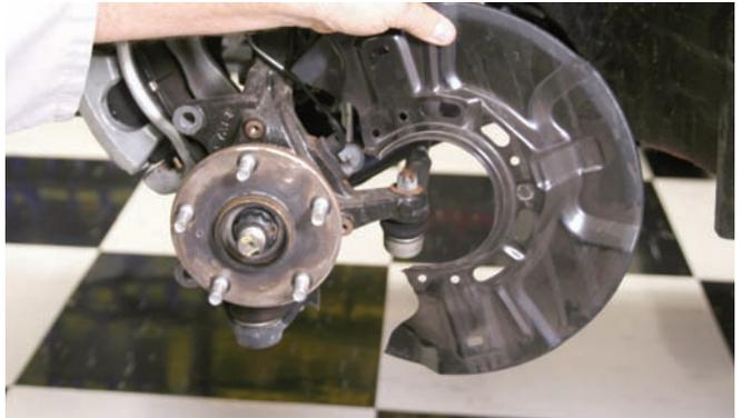
The dust shield was removed and it will not be used with the Wilwood brakes.
