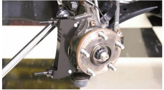
After the bolts were hand tight, they were tightened down with a large socket wrench. At this point they shouldn't be too tight because they may have to be loosened to add or subtract shims when the caliper to rotor centering is done. After the centering is complete, the bolts should be coated with Loctite 271 and tightened to 42 ft-lbs using a foot-pound torque wrench.
