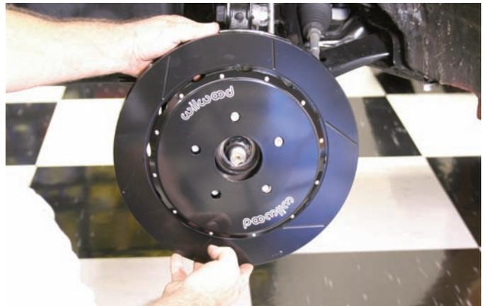
The hat was attached to the rotor using the 12 bolts and washers in the kit. The small bolts should be coated with Loctite 271 and then they should be tightened in an alternating sequence to 85 in-lbs using an inch-pound torque wrench. After the bolts were tight they were safety wired using the safety wire diagram in the instruction sheet. The completed rotor was installed on the hub assembly.
