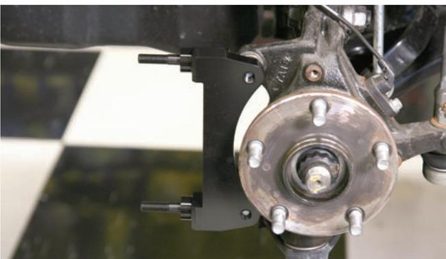
The caliper bracket was held against the original mounting ears and the bolts were installed hand tight.
