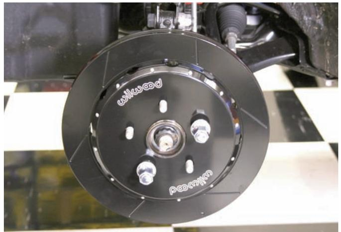
After the rotor was placed on the hub assembly, it was secured with two lug nuts in order to check the rotor to caliper centering.
