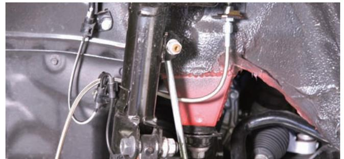
At this point the Wilwood part number 220-10803 hose assembly was installed. The hose runs from the bracket and hard line on the frame to the caliper assembly making sure the line is away from any moving parts.
