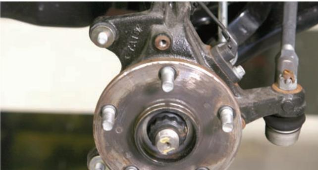
The caliper bracket bolts were installed in the mounting ears. There should be a washer on the outside and a 0.016-inch thick and a 0.030-inch thick washer between the original mounting ears and the caliper bracket.
