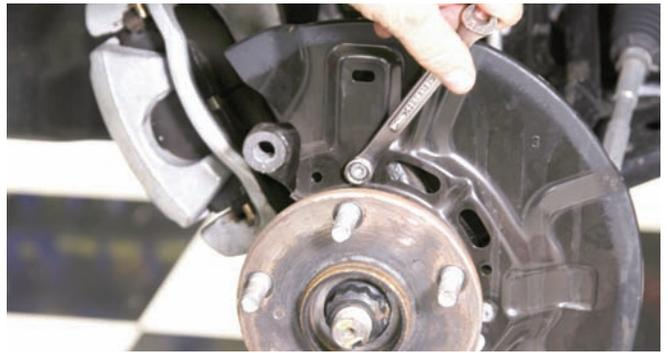
Using a small box-end wrench, the bolts that secure the dust shield to the spindle were removed.
