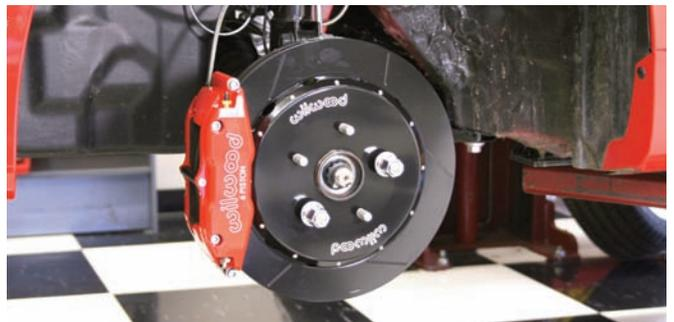
Here is the brake assembly finished and ready to go. At this point the brake system will have to be bled and the bedding process will have to be done to get the brakes working well and to full capacity.
