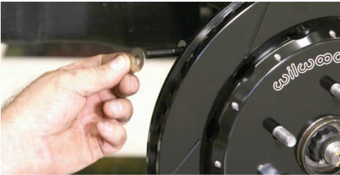
Before the caliper was installed on the caliper mounting bracket, each stud was loaded with a 0.035-inch shim.
