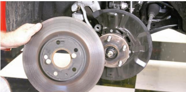
After the bolts were loose, the rotor was removed from the assembly. The rotor is in good condition so it can be stored with your other swap meet parts.
