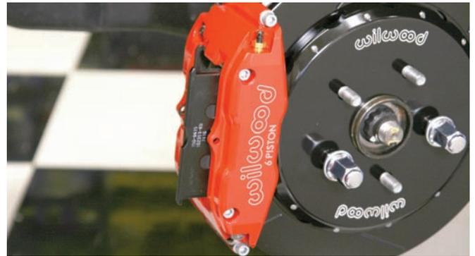
After the caliper was installed and tightened, the pads were installed from the top. After the pads were in place the caliper center bridge pad retainer bolt was installed.
