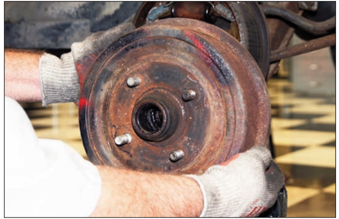
Sequence 4: Slide off the drum from the spindle. If it is stuck, it may be necessary to hit it a few times with a rubber mallet to break loose.
