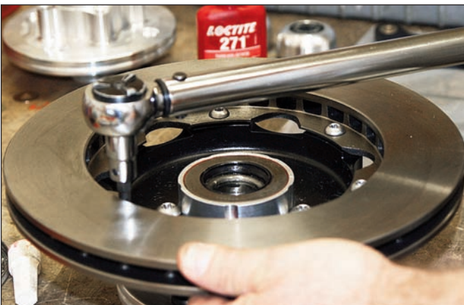
Sequence 14: Orient the rotor and the hat/hub assembly as shown above. Attach the rotor to the hat using supplied bolts. Using an alternating sequence, apply red Loctite® 271 to the threads, and torque to 25 ft-lb.
