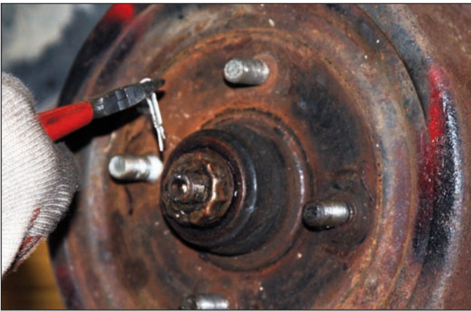
Sequence 2: Remove the dust cap, then the spindle nut retaining cotter pin, and nut lock.
