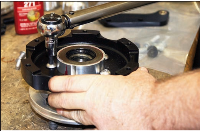
Sequence 13: Mount the hat to the hub using bolts as shown above. Using an alternating sequence, apply red Loctite® 271 to the threads, and torque to 55 ft-lb.
