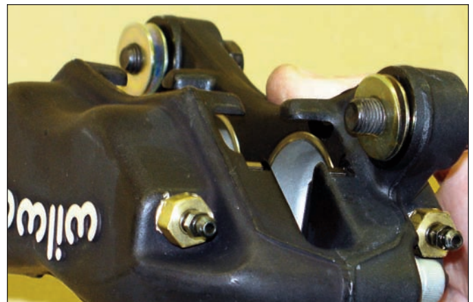
Sequence 17: Initially place two .035" thick shims on each bolt between the caliper and the bracket.
