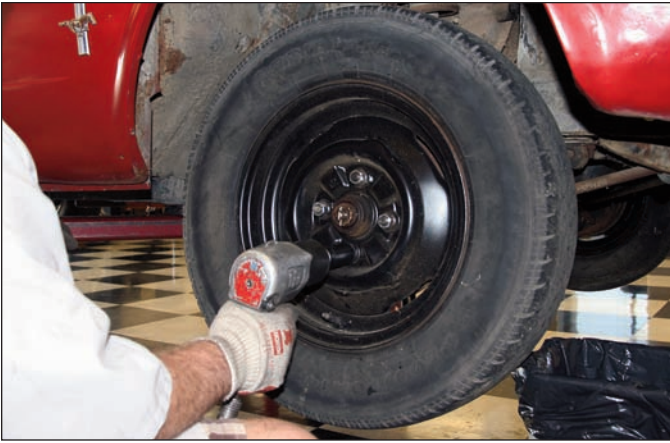
Sequence 1: Raise the front wheels off the ground and support the front suspension according to the vehicle manufacturer's instructions. Remove the lug nuts and remove the wheel.
