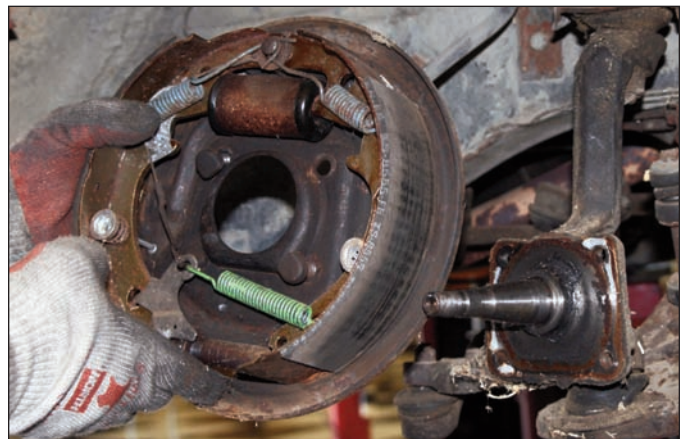
Sequence 6: Disconnect the brake hose at the chassis connection point and remove the drum brake assembly.
