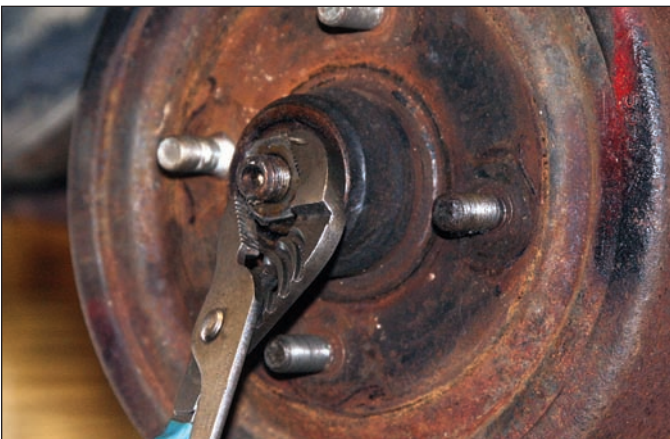
Sequence 3: Remove the spindle nut. Save the spindle nut and nut lock.
