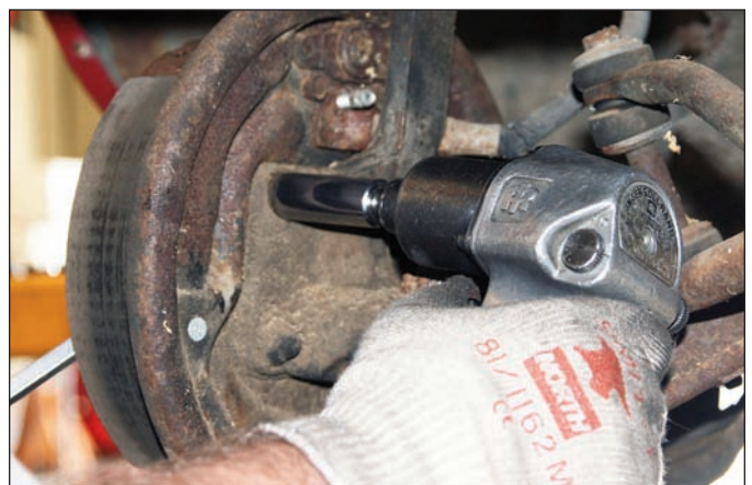
Sequence 5: Remove the bolts from the inboard side holding the drum brake assembly.
