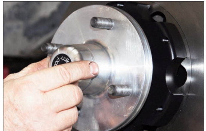
Sequence 16: Install dust cap into hub. Friction created by the o-ring on the dust cap keeps it from unscrewing. NOTE: The O.D. of the existing OEM spindle washer may be larger than the I.D. of the dust cap not allowing it to seat against the hub face. Therefore, use the spindle washer supplied with the kit instead of the OEM washer.
