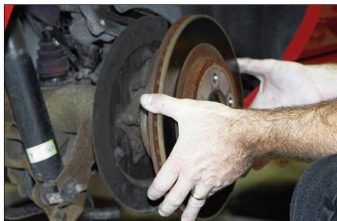
**Sequence 5:** Slide off the rotor from the hub. If it is stuck, it may be necessary to hit it a few times with a rubber mallet to break loose.
