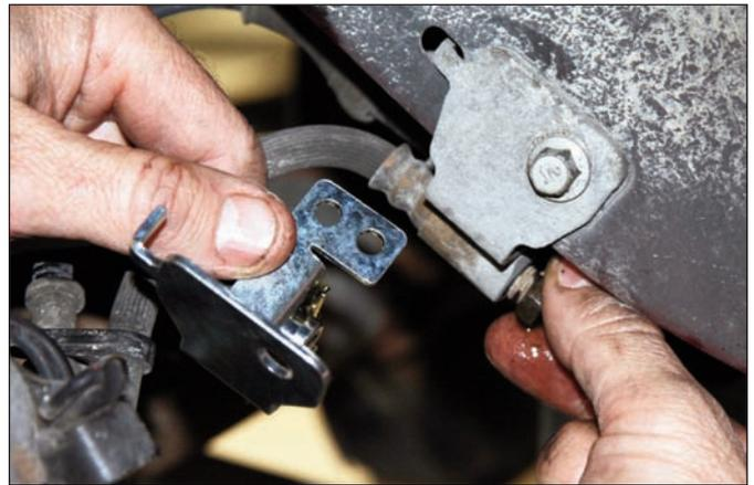
**Sequence 11:** Disconnect the OEM brake fluid hose where it connects to the brake hard line. Connect the new flexline to the hard line.
