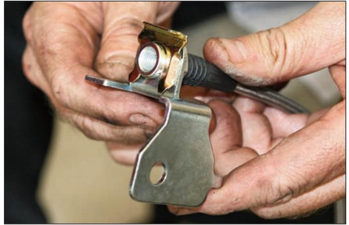
**Sequence 10:** Slip the new mounting bracket over the Wilwood flexline and secure with clip.
