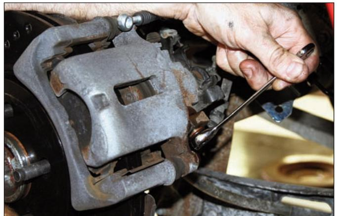
**Sequence 12:** Disconnect the other end of the rubber hose from the caliper. Try to keep fluid leakage to a minimum.
