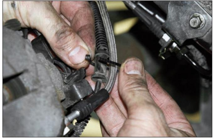
**Sequence 16:** Secure fluid line as necessary to prevent contact with moving suspension, brake, or wheel components. Bleed the system referring to the additional information in the data sheet as necessary for proper bleeding instructions.
