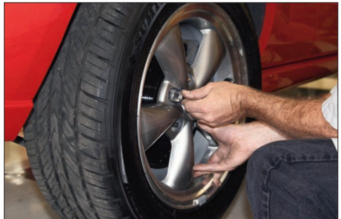
**Sequence 17:** Install the wheel and torque the lug nuts to manufacturer's specification. Rotate the wheel and check for any interference. Bed in the brake pads and rotor in a safe location before general use driving.
