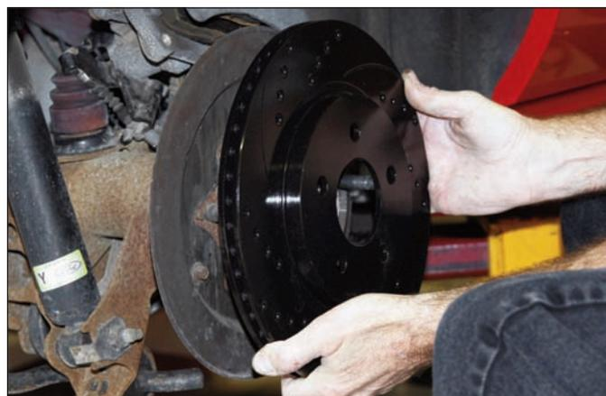
**Sequence 6:** Install the rotor over the hub assembly. **NOTE:** The rotor must fit flush against the axle hub flange or excessive rotor run out may result.
