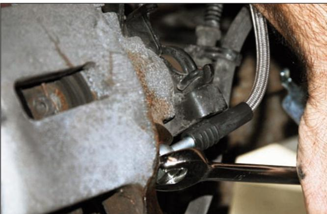
**Sequence 15:** Route line along the same path as the OEM hose and connect the other end of the flexline to the caliper.
