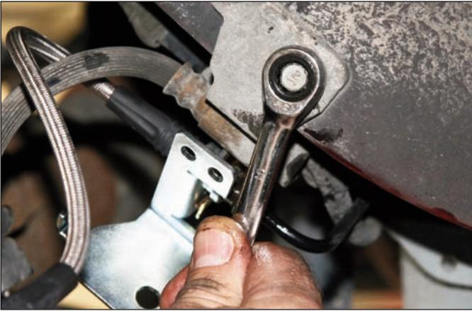
**Sequence 13:** Remove the old mounting bracket from the chassis. Save the mounting bolt.
